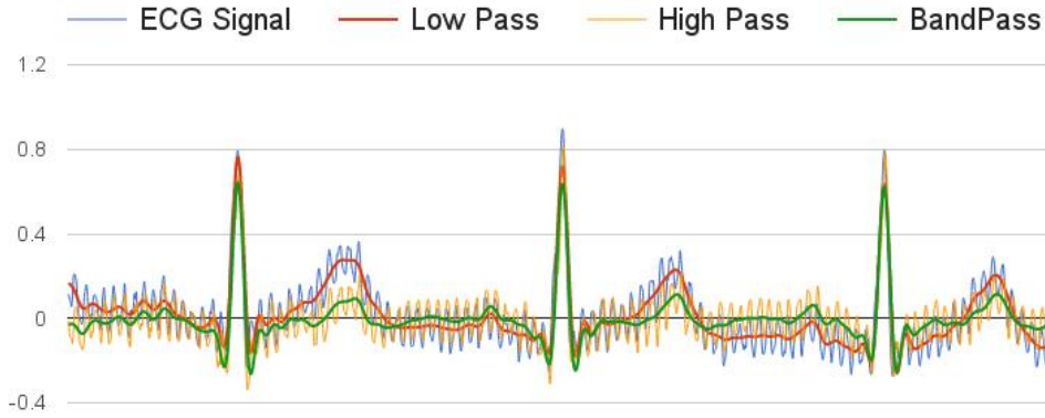
Fig.2. A segment of an ECG signal with several QRS complexes, filtered with a low pass filter of 30Hz, high pass filter of 0.5Hz and a band pass filter between 0.5Hz and 30Hz.
