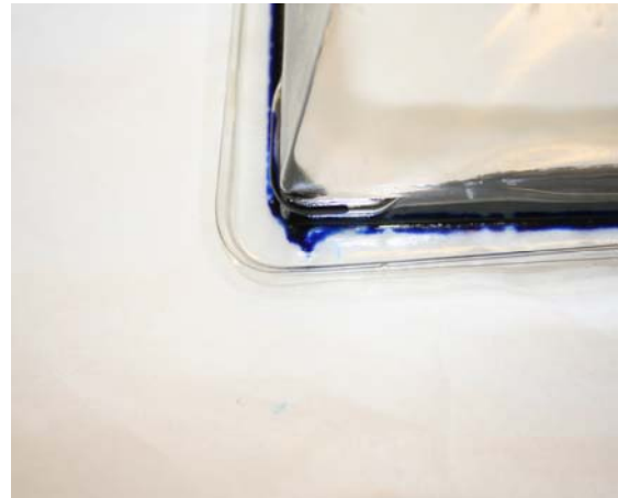
Figure 15 Poor control over seal area contamination caused this fault – the seal area had sauce on it.
