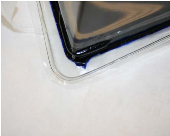
Figure 16 The two notches of blue ink matched exactly the damage seen on the sealing rubber.
