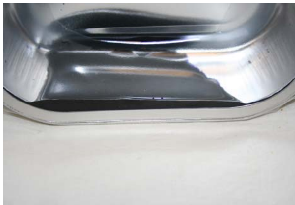
Figure 11 HFFS pack showing good seal integrity with a knurled sealing pattern. Some evidence of sealing rubber breakdown is evident in the corner of the pack
