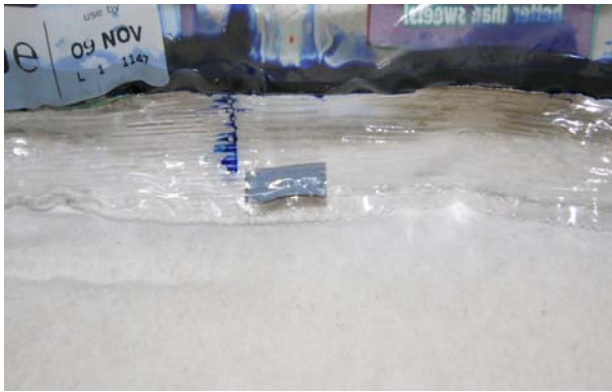
Figure 8 VFFS bag demonstrating that with adequate jaw pressure and correct settings even a major fold in the seal area will not necessarily leak.
