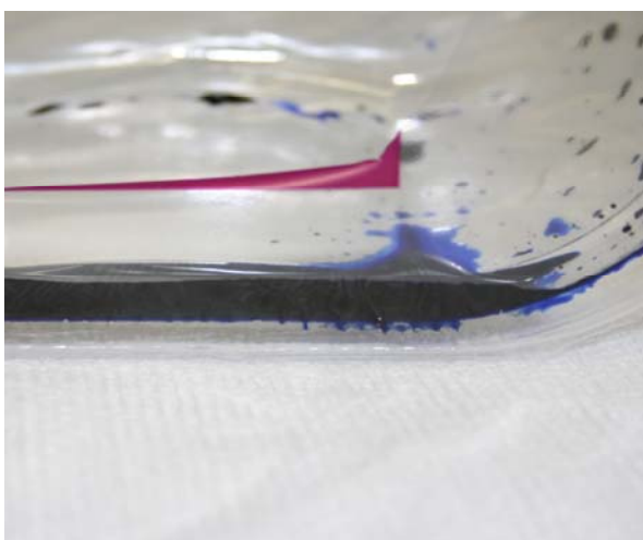
Figure 22 Some seal area contamination and cracked sealing rubber causing this faulty seal.
