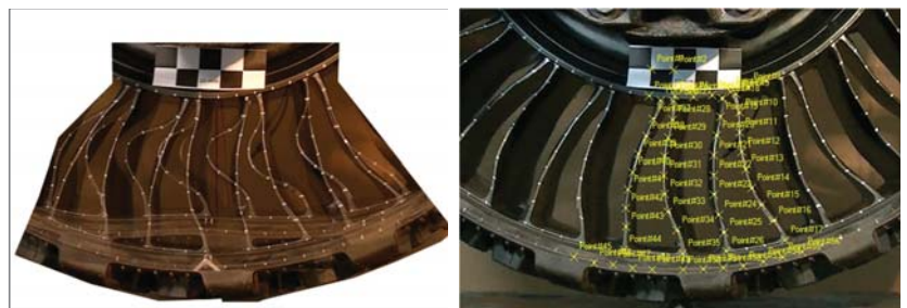
Figure 5. Summary of NPT_1 wheel images unloaded and loaded (image on the left), and preparation of reference points for the displacements analysis in the TEMA Automotive software (image on the right).
