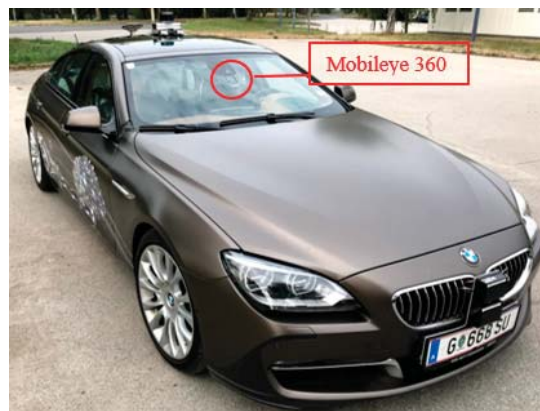
Figure 1. Testing vehicle with Mobileye 360 implemented behind the front windshield inside the vehicle.
