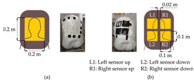
Figure 1. Sensors' configuration: (a) single sensor; (b) matrix sensor.
