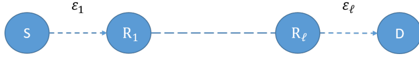
Figure 3.10: An example of an \ell -hop line network with loss rate \varepsilon_i per link, i \in \{1, \dots, \ell\} .
