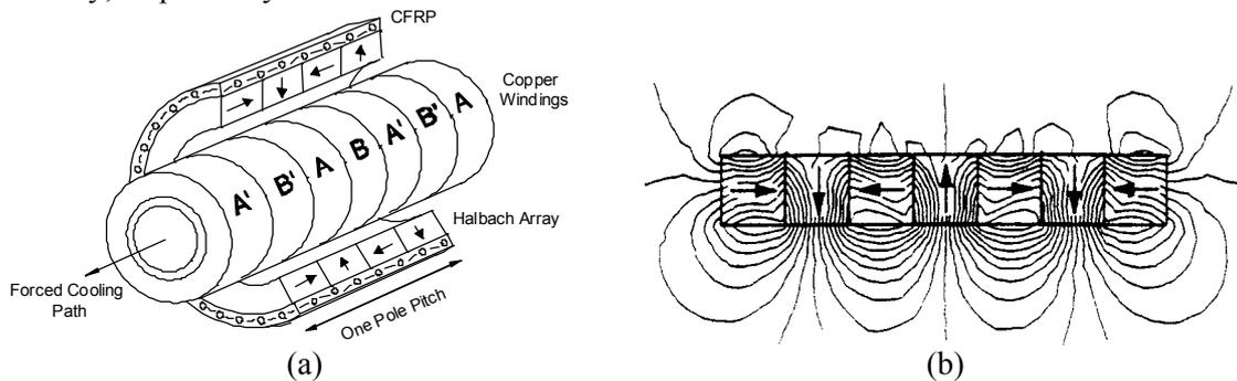
Fig.2: (a) 2-phase linear actuator with Halbach array (b) Self shielding Halbach array
