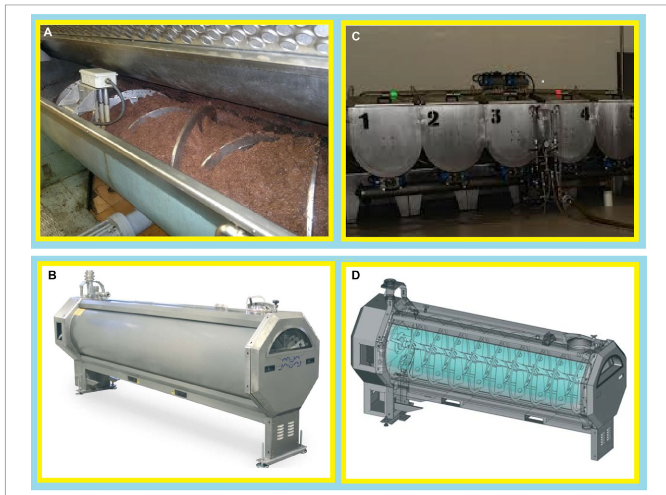
Figure 3—Malaxer machine and its evolution. (A) Traditional malaxing machine characterized by a cradle shape and a nonhermetic closure. This type of machine causes considerable loss of phenolic and volatile compounds. (B) Innovative malaxing machine characterized by a cylindrical jacket that covers the whole internal surface of the tank for a quicker and more efficient heating of olive paste. The hermetic sealing ensures a perfect control of the atmosphere in contact with the paste in the malaxing machine through valves for inert gas (nitrogen or argon) (photos courtesy of Alfa Laval, Olive oil SpA, Italy).
