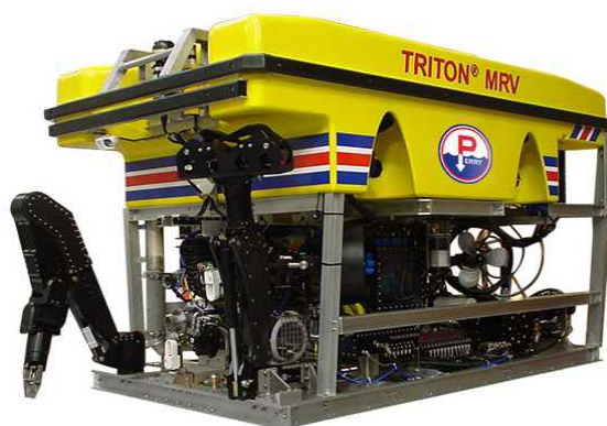
Figure 1. Deep-Sea (3000m) Remotely Operated Vehicle (ROV). (Photograph courtesy of Perry Slingsby 1 )
