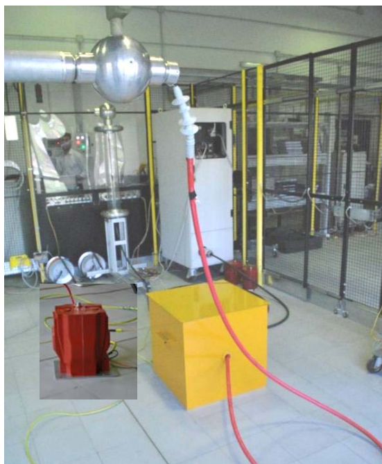
Figure 6. Voltage calibration with the divider inside a metallic grounded box.
