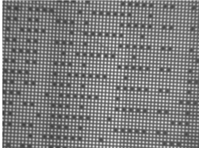
Figure 3.13: Image of a local area of Pseudo-Periodic Pattern (PPP) where every dot is 2 \mu m in diameter.
