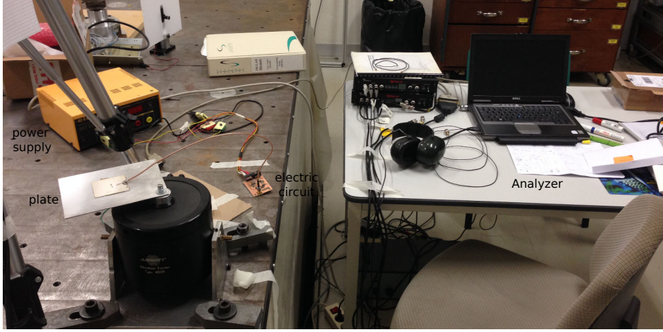
Figure 3.7: Layout measurement system for a single patch.
