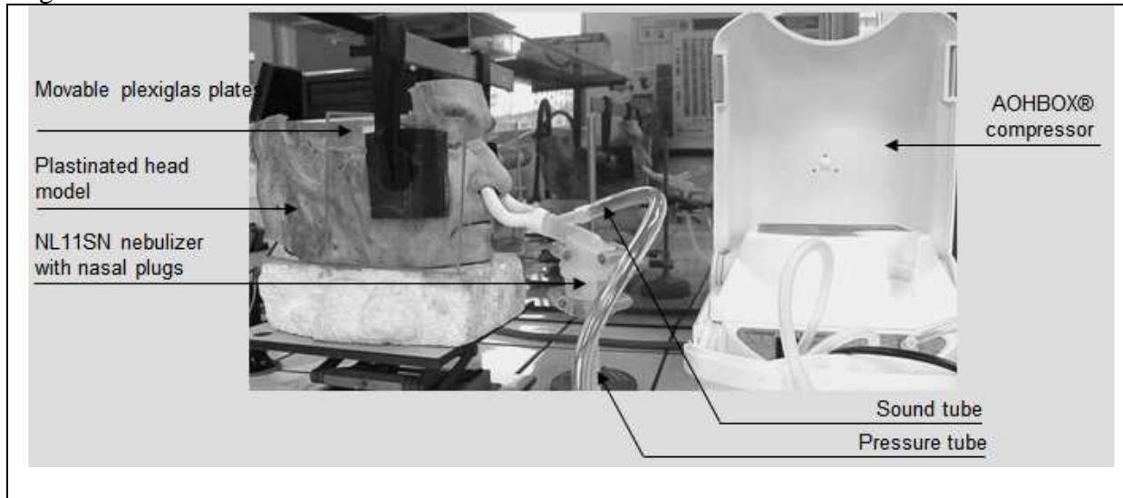
Figure 1: Nebulization of gentamicin in a plastinated head model, using the ATOMISOR NL11SN nasal sonic nebulizer connected to an ATOMISOR AOHBOX® compressor.
