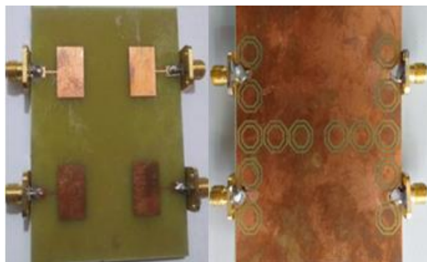
Figure 9 A fabricated proposed MIMO Antennas top and bottom view
