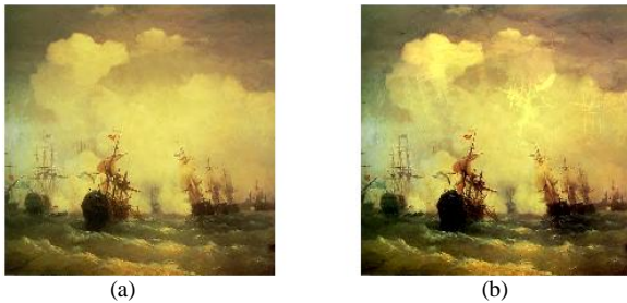
Figure 17. (a) The original color image and (b) the image enhanced channel-wise by the 2-D EDFTs with angles \phi_1 = \pi/6 and \phi_2 = \pi/4 .
