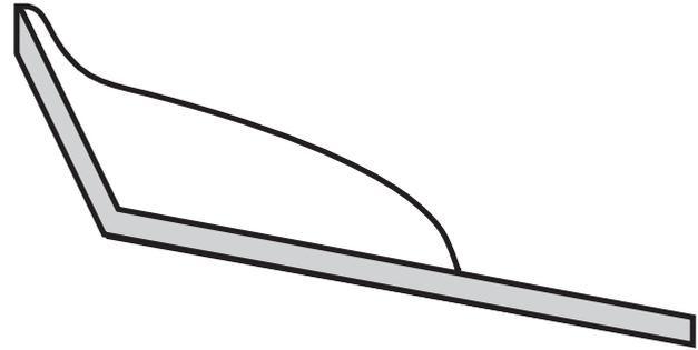
**Fig. 1.** Schematic view of the glacier considered in the two-layer model. The ice body (white) resides on a sediment layer (grey) which extends into the glacier forefield. The inclination of the upper part is  $45^\circ$  and of  $5^\circ$  for the lower part.
