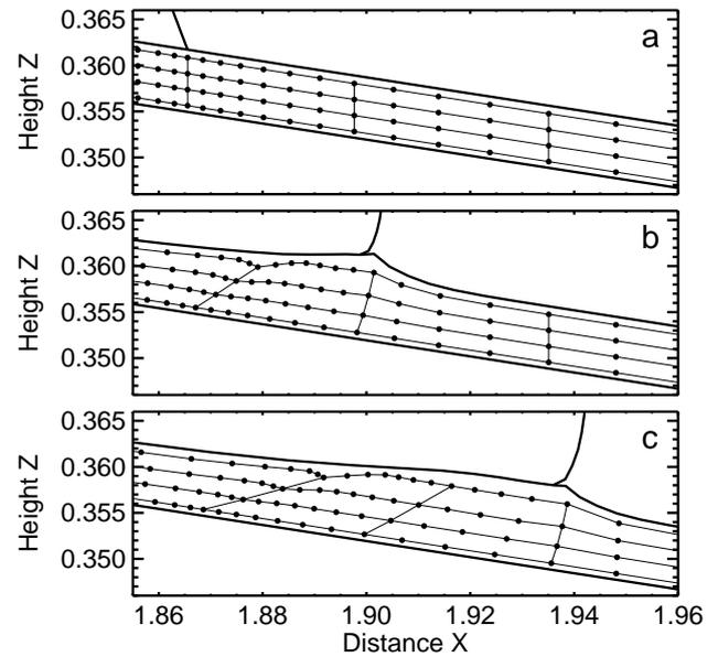
**Fig. 12.** Experiment C: Moderately stiff and moderately non-linear till ( $m = 3$ ,  $B = 0.79$ ): Sediment layers which were originally parallel to the bed (a) are deformed and form a wave to keep the sediment bulge in position (b–c). The snapshots were taken at dimensionless times  $T$  equal to 0 (a), 8 (b) and 14 (c). Three vertical straight lines in (a) are followed throughout (b–c).
