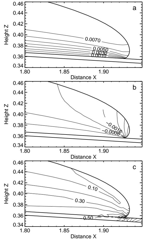
**Fig. 8.** Experiment A: Relatively stiff and moderately non-linear till ( $m = 3$ ,  $B = 8$ ): Snapshots at dimensionless time  $T = 15.4$  showing the distribution of horizontal velocity (a), vertical velocity (b) and effective stress (c) in the frontal part of the glacier. Note that the effective stress in the sediment is decreasing distal of the glacier front.
