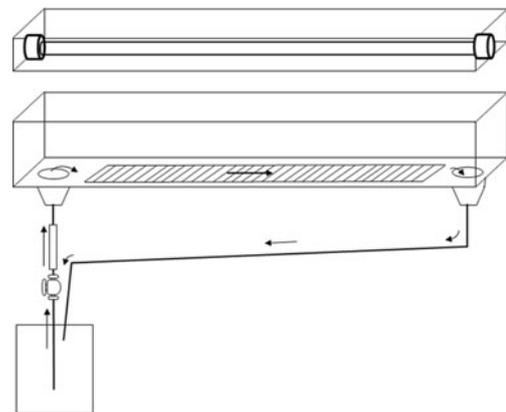
**Fig. 1** Scheme of a chamber of the continuous flow-lane incubator prototype used to culture biofilm-forming cyanobacteria strains. A flow channel through medium circulated over a surface covered with polycarbonate slides. Each chamber contained the light source and the circulation of culture medium could be regulated. See text for details
