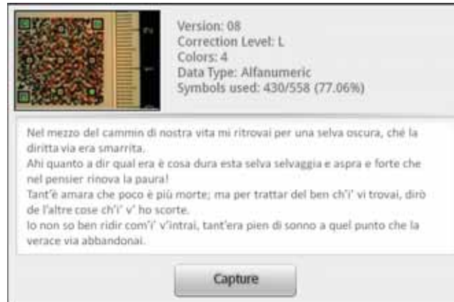
Fig. 11. A sample screen shot involving a successfully decoded 4-color HCC2D code (version 8). Printout size: 1x1 inches. Device: HTC Hero, running Android 2.1.
