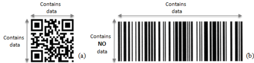
Fig. 1. Dimension for storing data in (a) 2D and (b) 1D codes.
