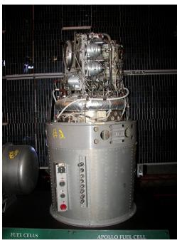
Figure 1.11 Apollo Fuel Cell Simulator
