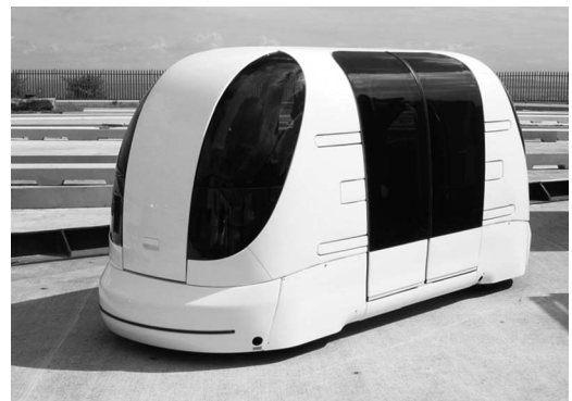
Fig. 1. ULTRA PRT vehicle [1].
