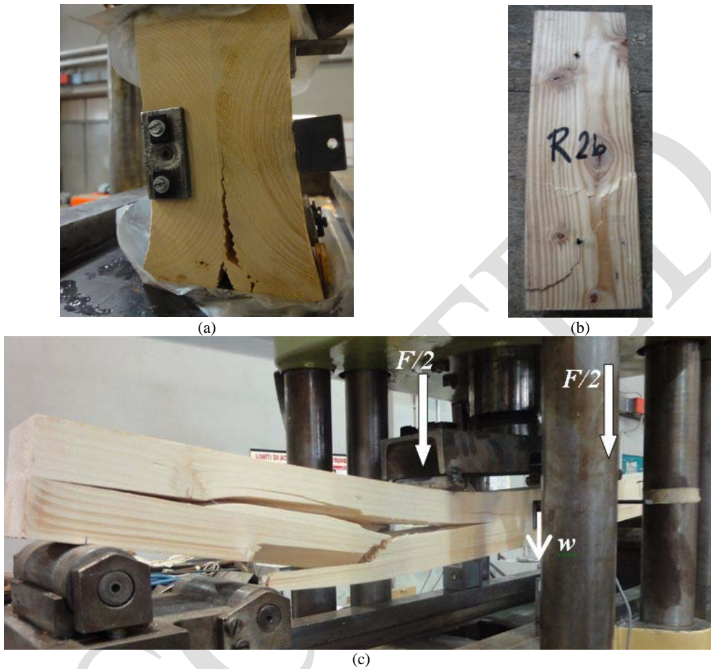
Fig.22. Experiments on small Blockhaus specimens. Failure configurations for (a) 'Tirol' log samples and (b) rounded dovetail samples. (c) Bending experiments for the estimation of the longitudinal shear modulus G .
