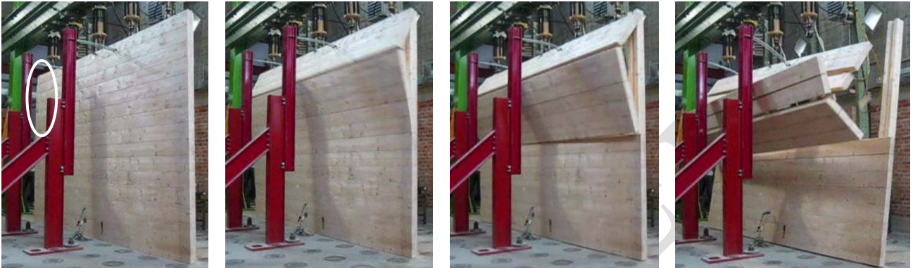
Fig.17. Collapse mechanism of specimen W05. Sequence of progressive cracking. In the circle, the area of crack initiation.
