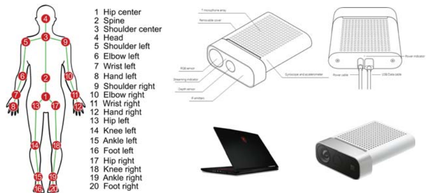
Figure 5. Microsoft Azure Kinect DK™ basic tracking capabilities and internal hardware architecture. A laptop computer that integrates a Nvidia graphics card must be used to fully take advantage of the tracking module.
