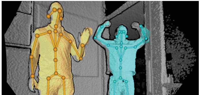
Figure 2. Graphical representation of the data collected by the tracking device. Multiple skeletons can be simultaneously tracked.
