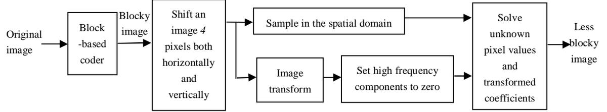
**Fig. 1.** Block diagram of the proposed de-blocking technique
