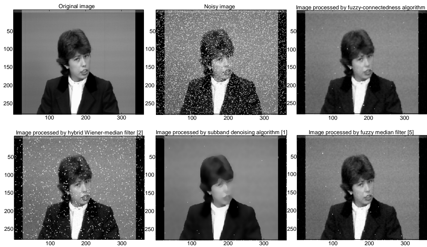
Fig. 5. Simulation results of corrupted video signal Claire processed by different algorithms
