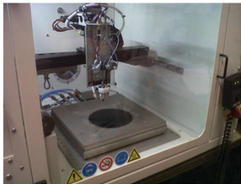
Fig. 109 Photograph of a catalytic ink printer used to spray catalytic inks onto PFSA membranes (batch process, lab-scale). Reproduced with permission from Paris-Saclay University.
