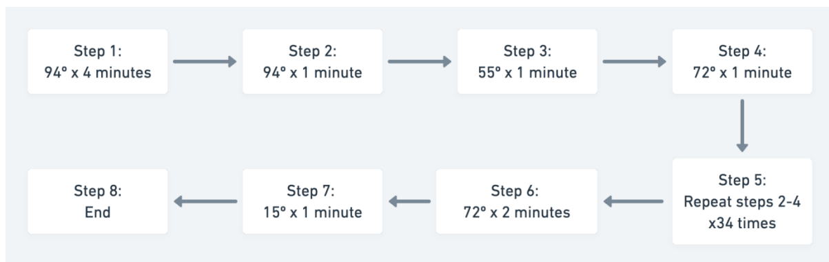
Figure 6.7: A flow chart of the thermal cycler settings and steps
