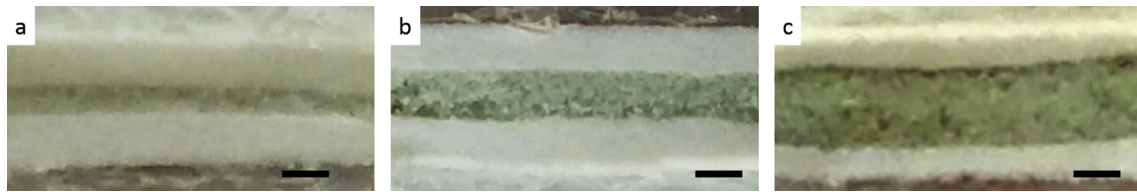
Fig. 5. Digital photo of sections of the multi-phasic laminates with the PLA core layer green colored. a) PCL laminate with PLA core 0.5 mm thick (LAM_0.5); b) PCL laminate with PLA core 1 mm thick (LAM_1); c) PCL laminate with PLA core 2 mm thick (LAM_2). Scale bar is 1 mm. (For interpretation of the references to colour in this figure legend, the reader is referred to the web version of this article.)
