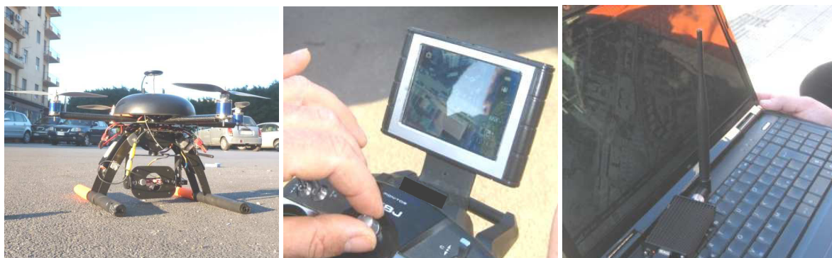
Fig. 1. Equipment employer for video recording: UAV with video camera (a), remote control (b) and ground control station (c). In the table 2 there are the micro-drone technical features.
