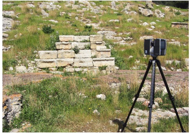
Figure 2. Laser scanner survey
