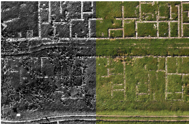
Figure 9: Visual check between the ortho images made with PhotoScan (in B&W) and made with Socet Set (in RGB)
