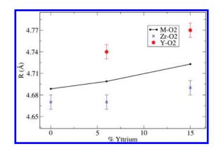
**Figure 13.** Comparison of fourth shell Zr–O, Y–O, and M–O distances probed by XRD and EXAFS as a function of  $Y^{3+}$  content in hydrated BZY samples.
