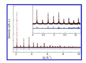
Figure 3. XRD data and model for BZY6HYD.
