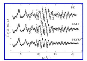
Figure 4. Zr K-edge EXAFS data (circles) and best fit (thick line) of hydrated BZY samples.
