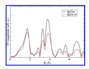
Figure 9. Comparison of Fourier-transformed Y K-edge EXAFS data of hydrated BZY samples.
