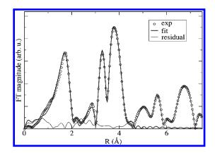
Figure 7. Fourier-transformed Y K-edge EXAFS data (circles), best fit (thick line), and residual (thin line) of BZY6HYD.
