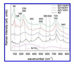
**Figure 14.** Raman spectra of dry BZY samples with different Y-content, along with the spectrum of undoped SrTiO<sub>3</sub>. Pink dashed lines: phonon modes for cubic SrTiO<sub>3</sub>.
