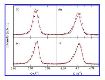
**Figure 1.** Comparison of the XRD best fitting for BZY15HYD, obtained with cubic (panels a and b) or tetragonal (panels c and d) models. The two peaks correspond to the (200) and (310) reflections of the cubic unit cell, respectively.
