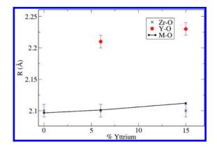
**Figure 10.** Comparison of first shell Zr-O, Y-O, and M-O distances probed by XRD and EXAFS as a function of  $Y^{3+}$  content in hydrated BZY samples.
