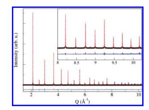
Figure 2. XRD data and model for undoped BZ.
