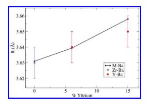
Figure 11. Comparison of second shell Zr–Ba, Y–Ba, and M–Ba distances probed by XRD and EXAFS as a function of  $Y^{3+}$  content in hydrated BZY samples. Note that for BZY6 and BZY15, the Zr–Ba symbols and error bars are covered by Y–Ba.
