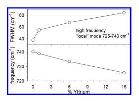
**Figure 16.** Variation of the position and width of the Raman peak at 740  $\text{cm}^{-1}$  as a function of dopant content.
