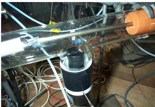
Figure 6: Townson and Mercer temperature chamber.
