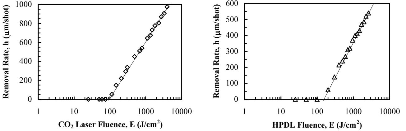
Fig. 1. Removal rate per shot,  $h$ , as a function of (a) CO<sub>2</sub> and (b) HPDL laser fluence,  $E$ .
