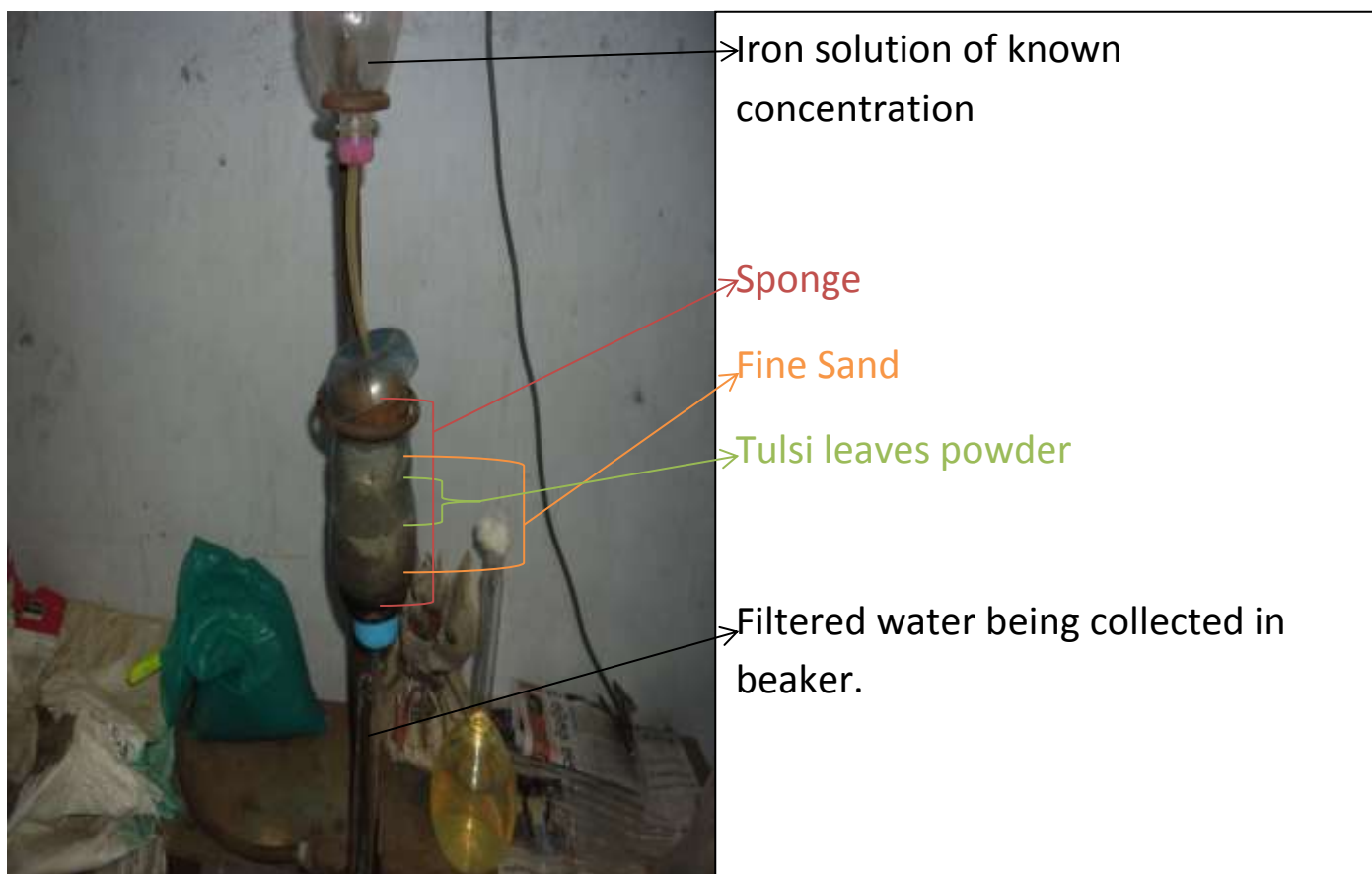
Fig4.1 Filtration with Tulsi leaf powder
