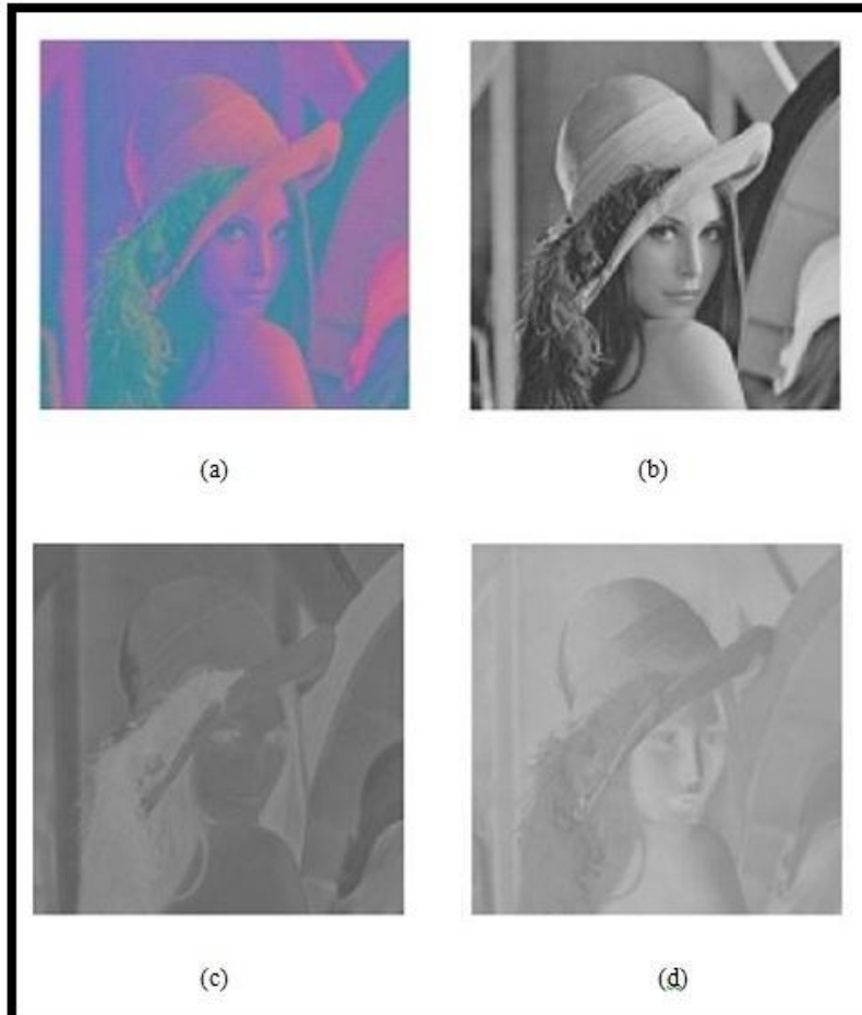
Figure 2.3: (a) Lena image represented in the YCbCr color space. (b) Luminance component. (c) Chrominance-red component. (d) Chrominance-blue component.
