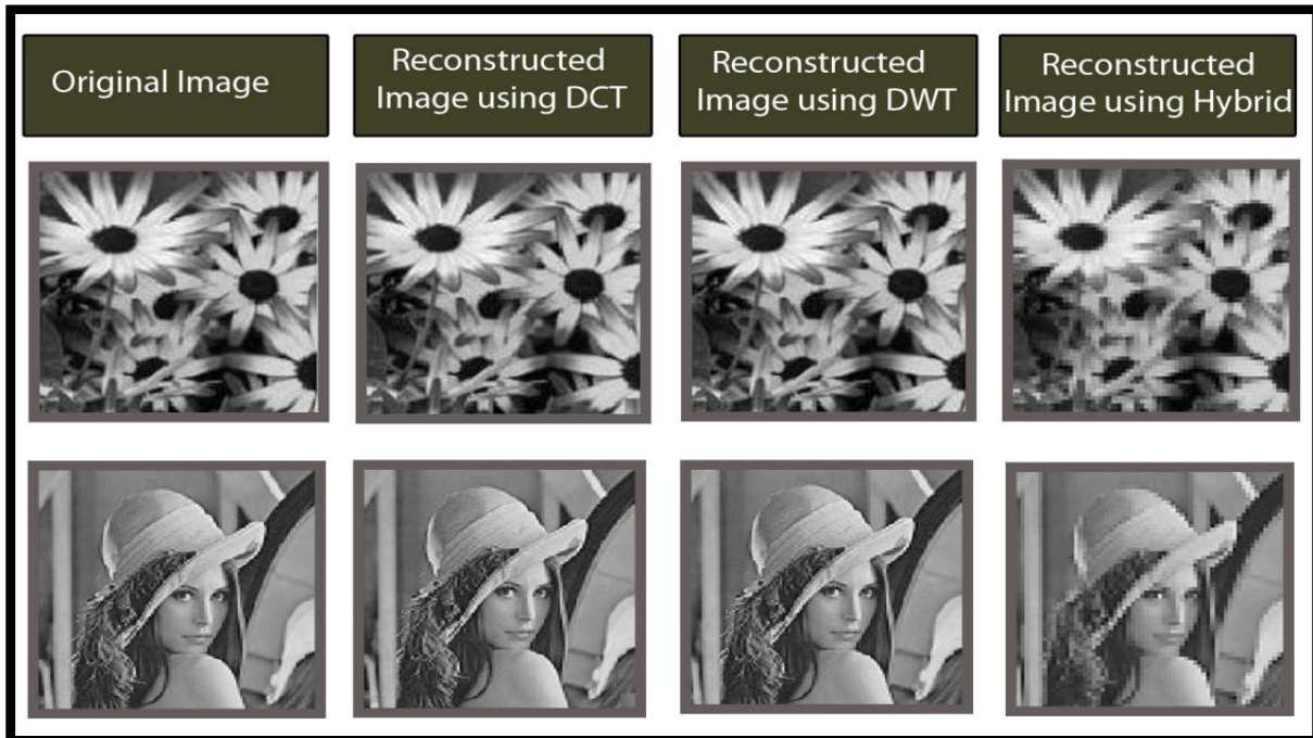
Figure. 4.1 Comparison of visual image quality of reconstructed image for DCT, DWT AND HYBRID (DCT+DWT) for test images.
