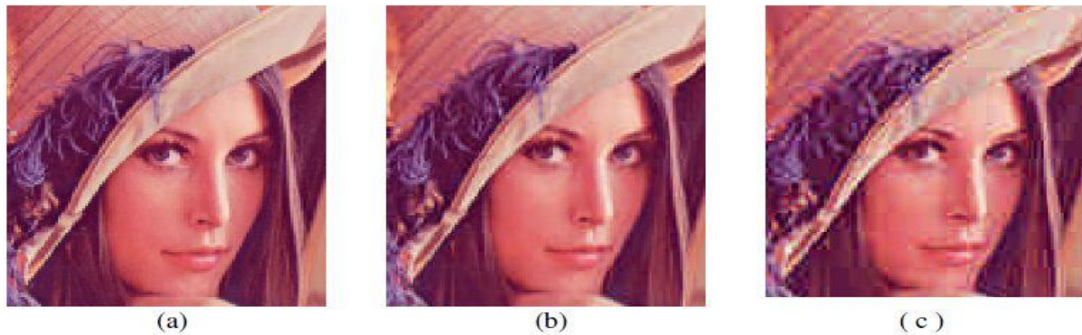
Figure 2.17. Illustration of compression using DCT: (a) Original Image CR at (b) 88%, (c) 96%
