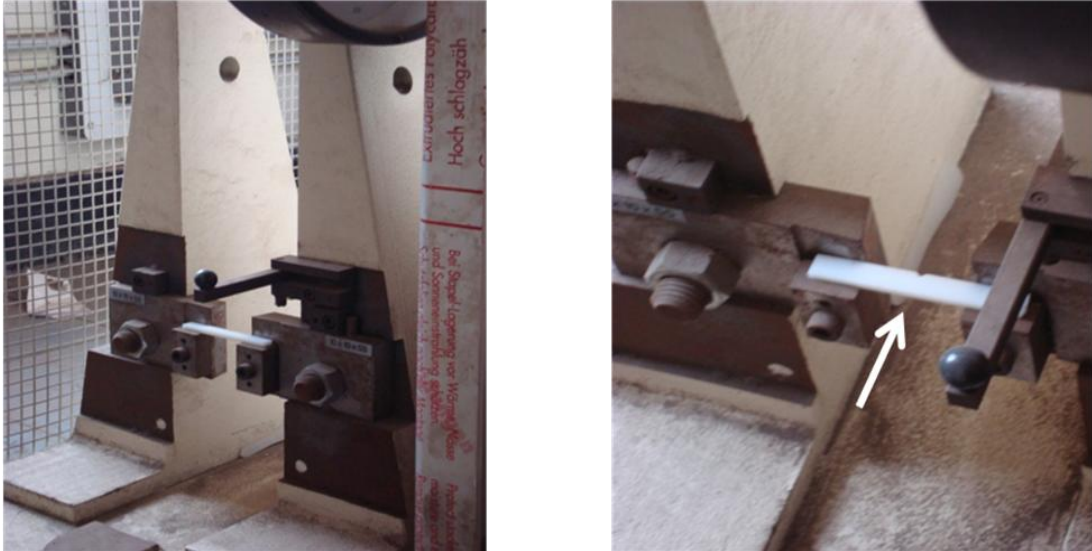
Figure 3.12 Instron Wolpert pendulum impact test machine (arrow shows direction of impact)
