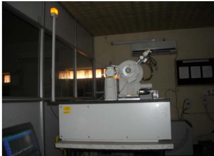
Fig.3.4: PANalytical system diffractometer (Model: DY-1656).
