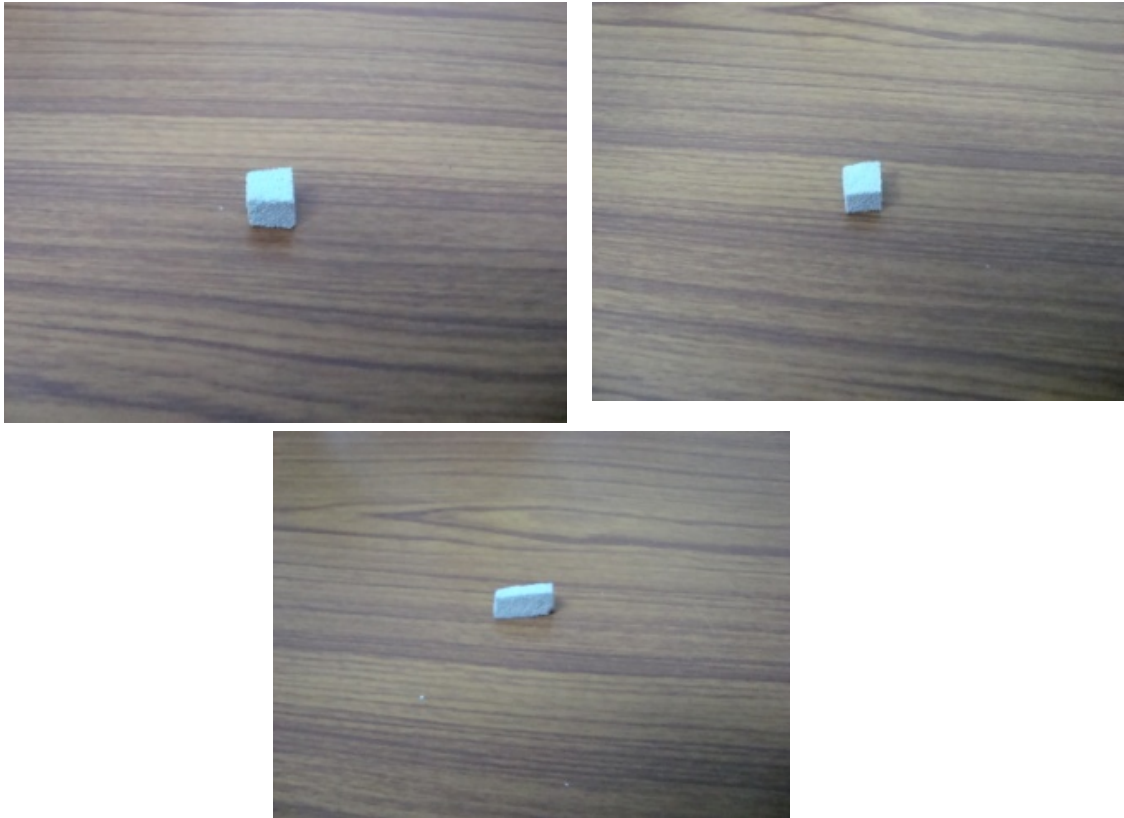
Fig-4.2 sintered hydroxyapatite scaffold prepared by polymeric sponge method.
