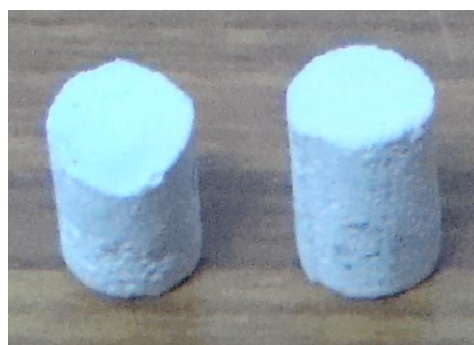
Fig-4.3 PEG-HAP scaffold sintered at 1250°C
