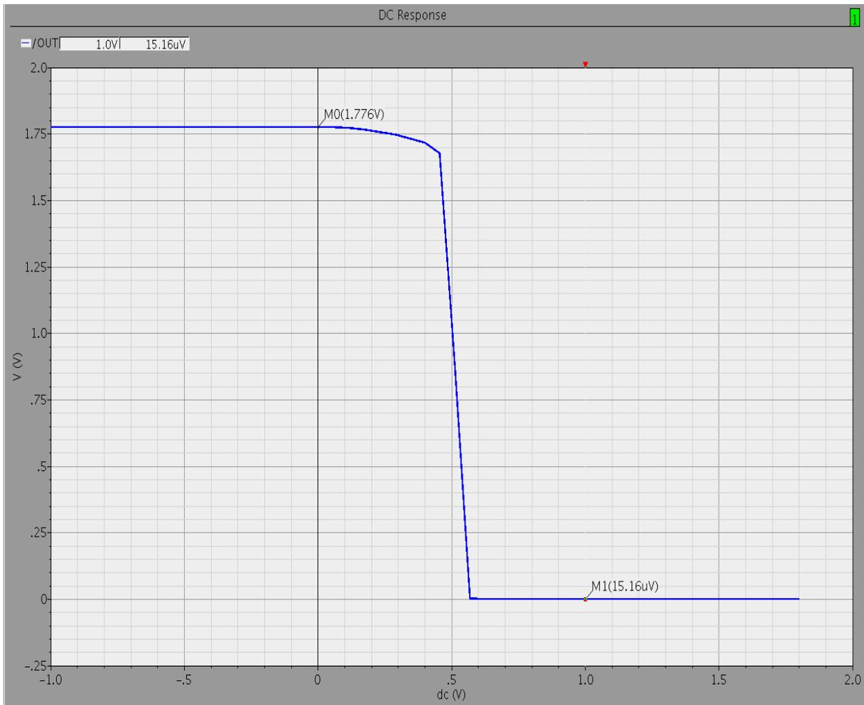
Fig. 4.8 DC Waveform for dynamic comparator using positive feedback
