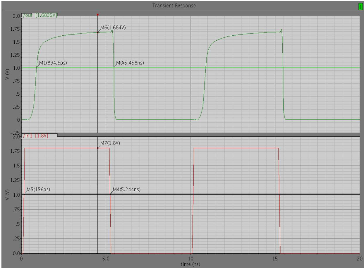
Fig. 3.15 Transient analysis waveform for Differential Dynamic Comparator
