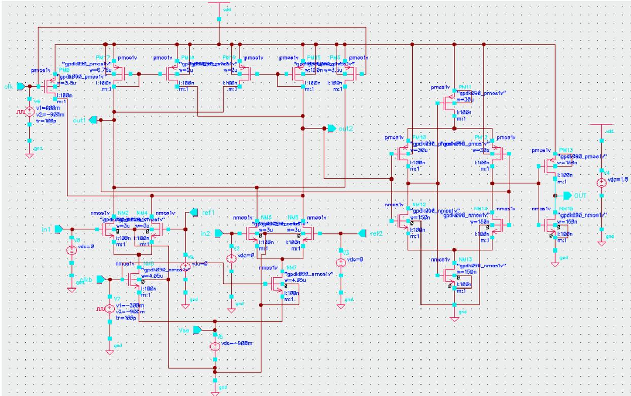
Fig. 4.9 Offset circuit for dynamic comparator using positive feedback
