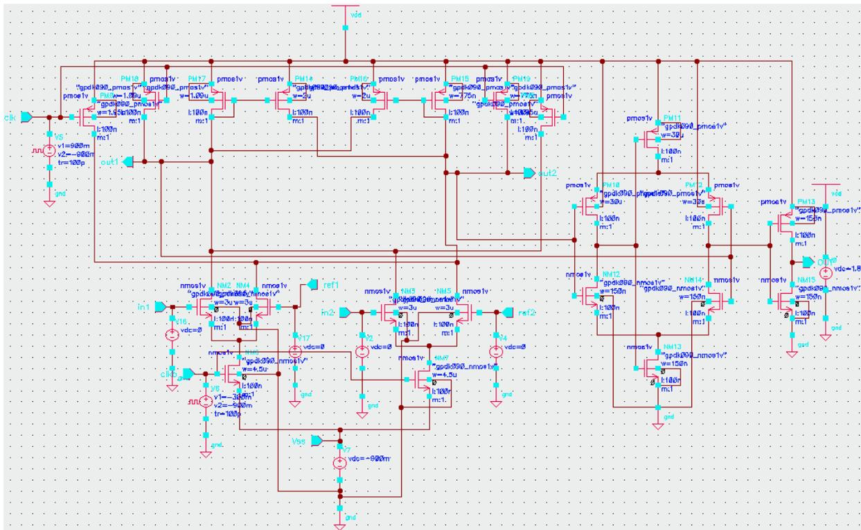
Fig. 4.15 Offset Circuit for dynamic comparator PMOS as switch
