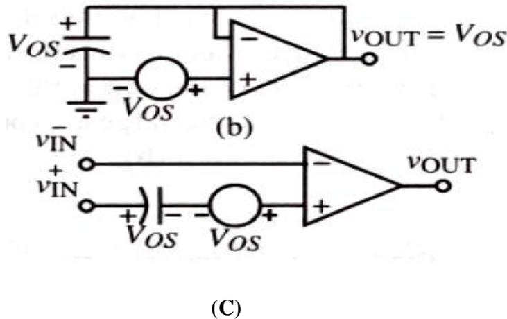
2.11 (b) Comparator during phase  $\phi_1$ , 2.11(c) Comparator during phase  $\phi_2$
