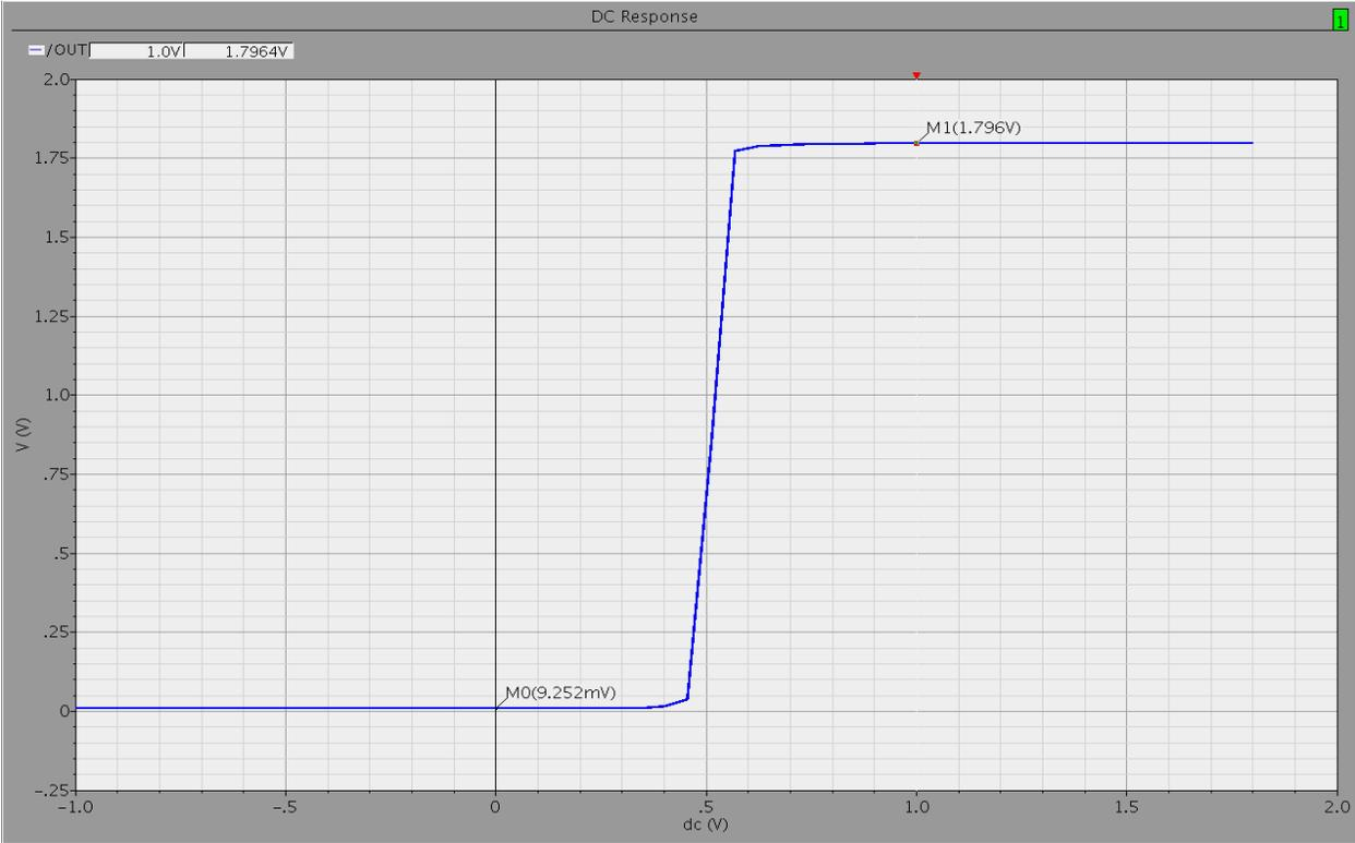
Fig. 3.11 DC Response of differential dynamic comparator
