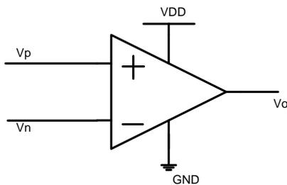
$$V_P < V_N \text{ then } V_O = V_{SS} = \text{logic } 0.$$
