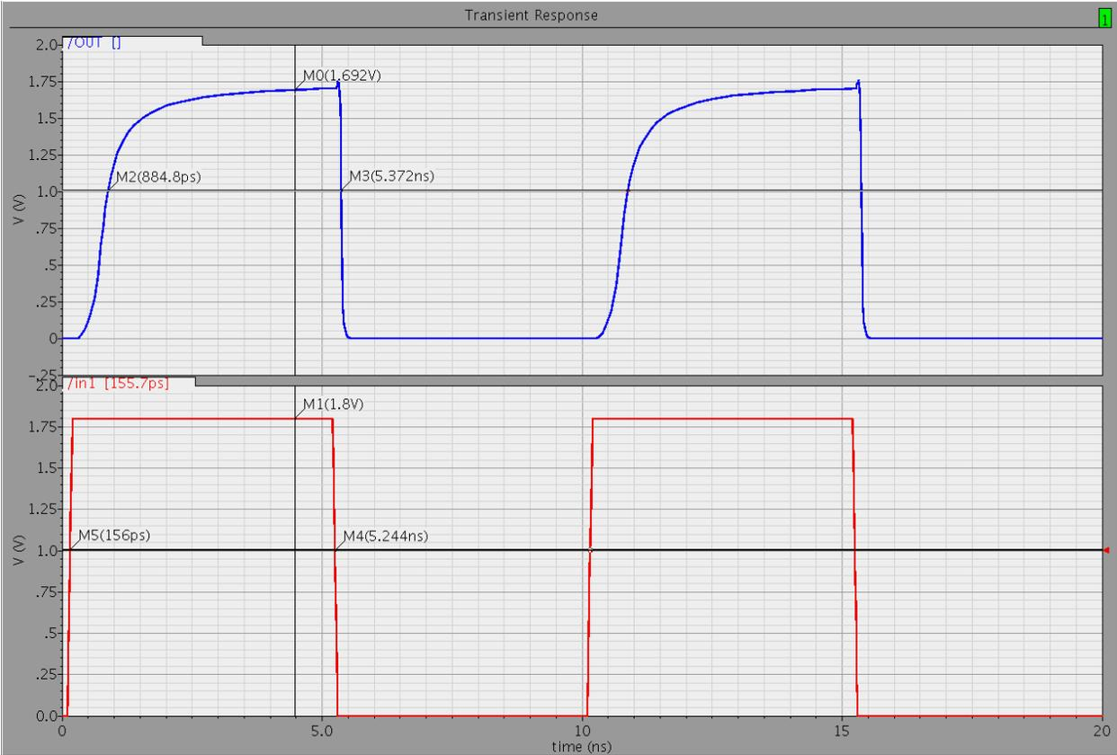
Fig. 4.12 Transient wave form for dynamic comparator using positive feedback
