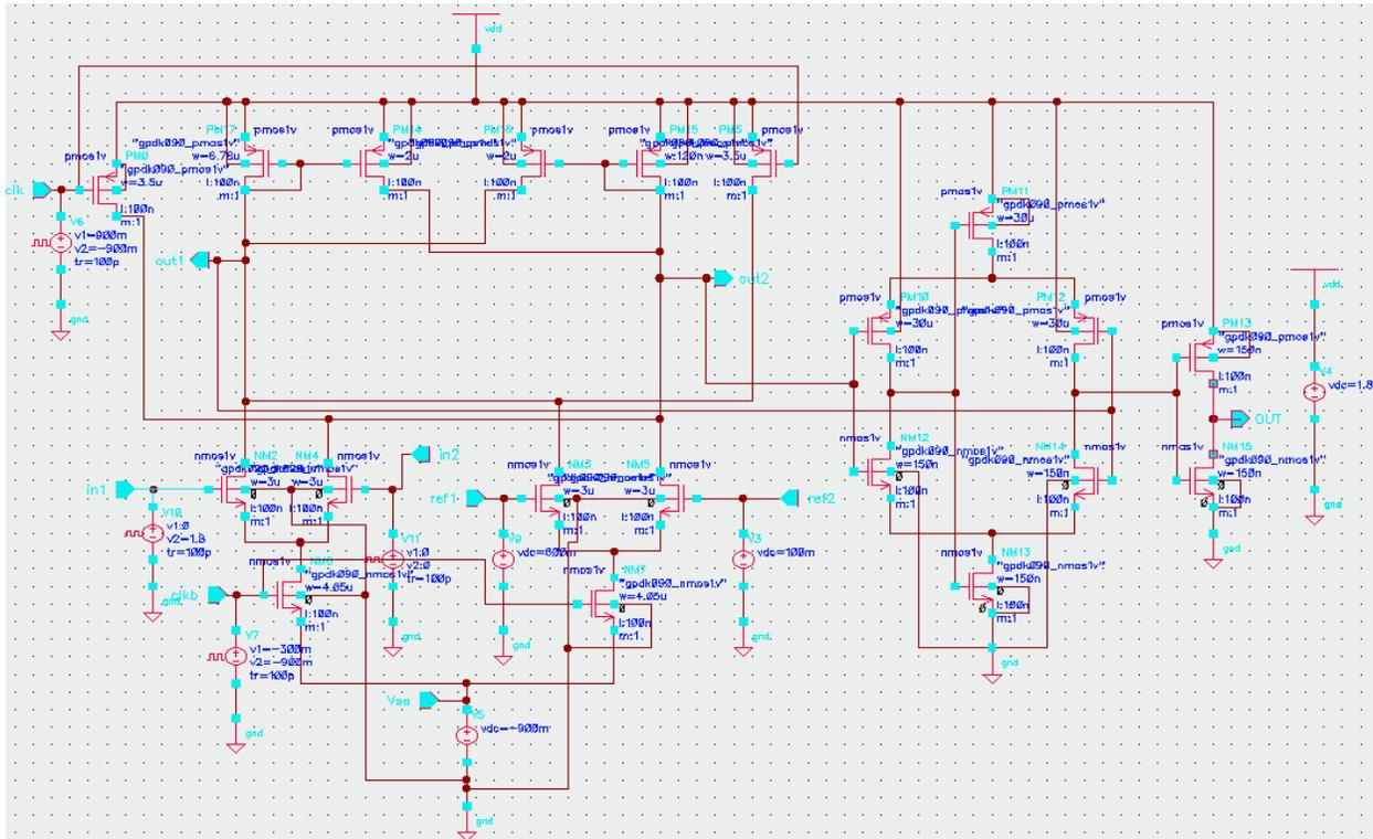
Fig. 4.11 Transient circuit for dynamic comparator using positive feedback
