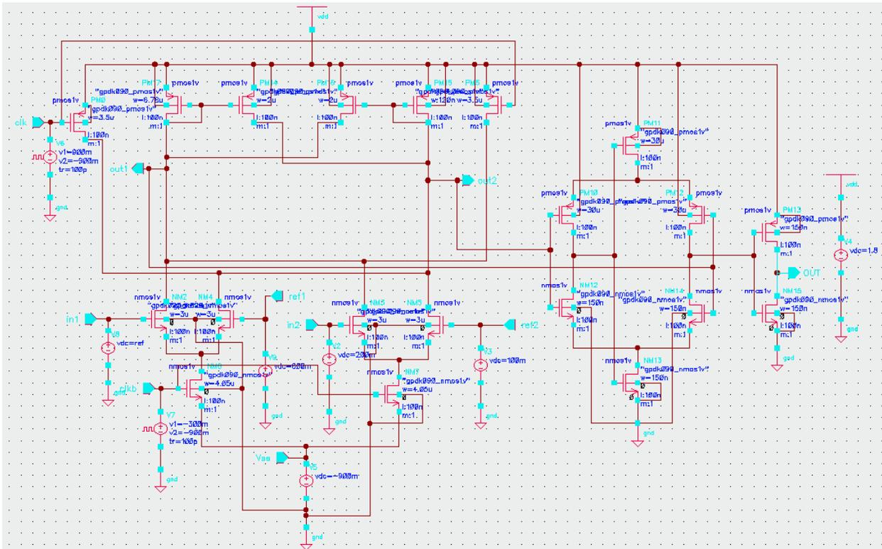
Fig. 4.7 dc circuit dynamic comparator using positive feedback
