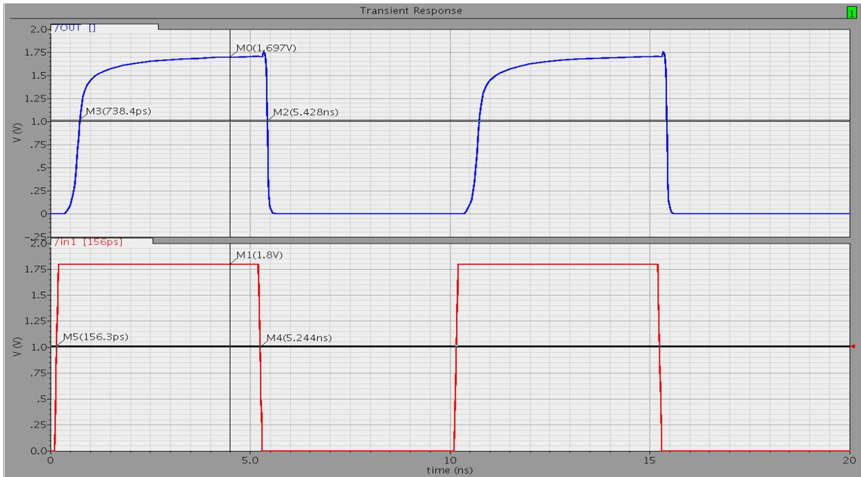
Fig.4.4 Transient response of dynamic comparator
