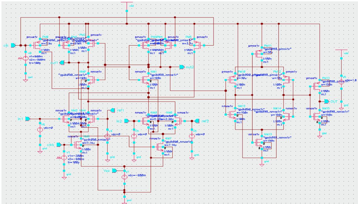
Fig.4.5. Offset voltage circuit for dynamic comparator
