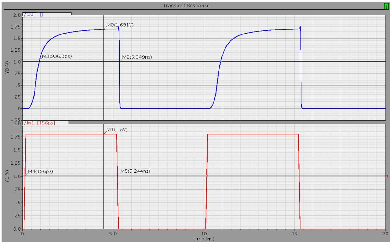
Fig. 4.18 Transient wave form for dynamic comparator PMOS as switch
