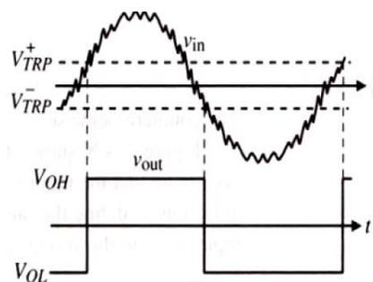
2.12 (c) Comparator response to a noisy Input when hysteresis is added
