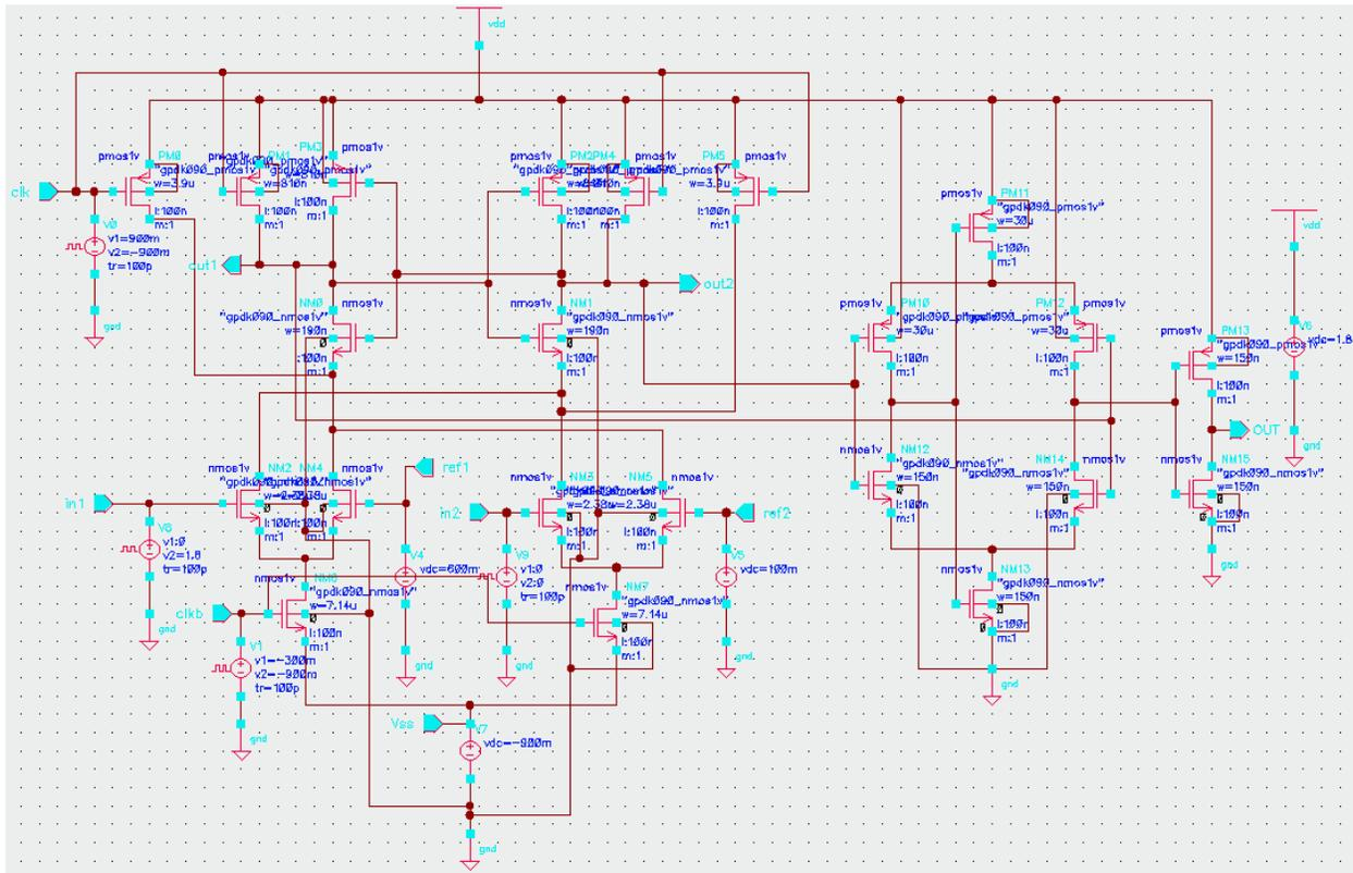
Fig.4.3 Dynamic comparator transient response circuit
