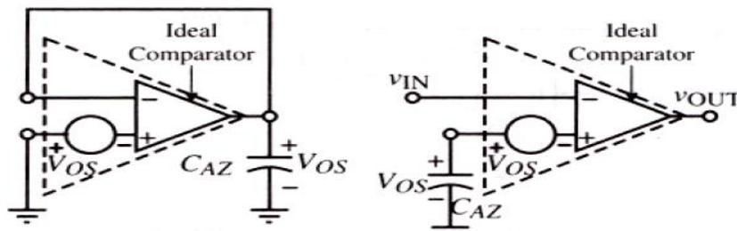
2.10 a) Comparator unity-gain configuration storing the offset on auto zero capacitor  $C_{AZ}$  during first half of the auto zero cycle. 2.10 b) Comparator in open-loop configuration offset cancellation achieved at the non inverting input during the second half of the auto zero cycle.
