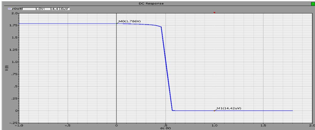
Fig. 4.14 DC Waveform for dynamic comparator PMOS as switch
