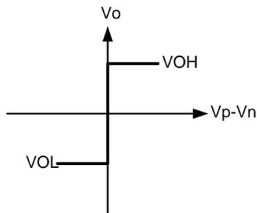
**Fig.2.1. Ideal transfer curve of a Comparator**
