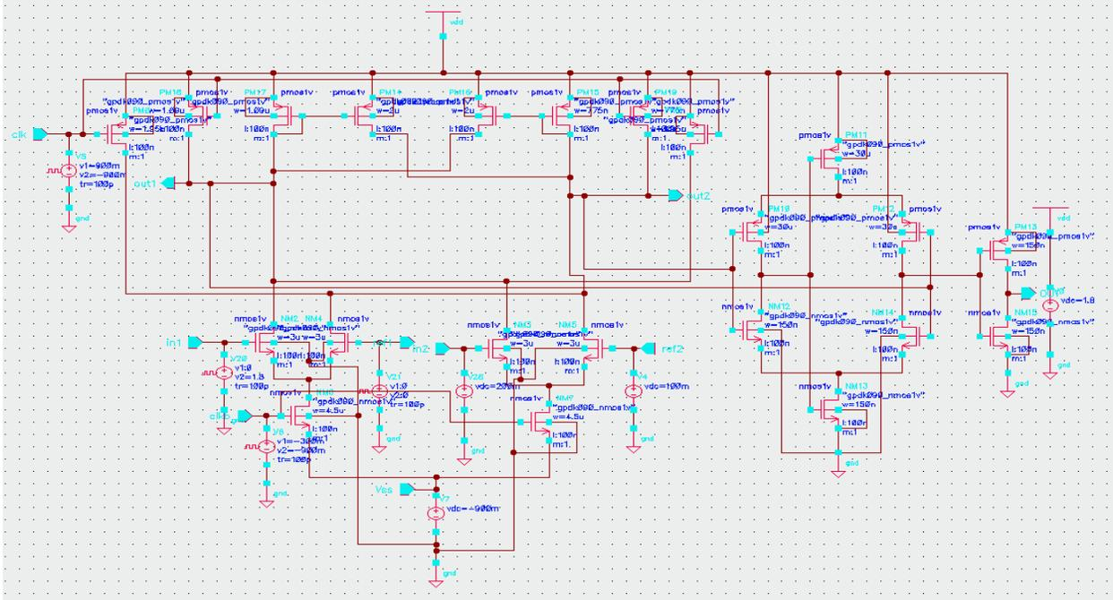
Fig. 4.17 Transient circuit for dynamic comparator PMOS as switch
