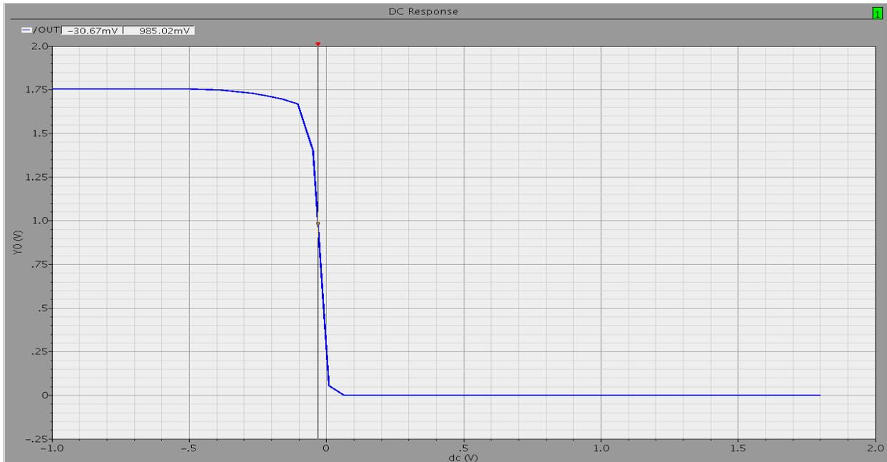
Fig. 4.10 Offset Waveform for dynamic comparator using positive feedback
