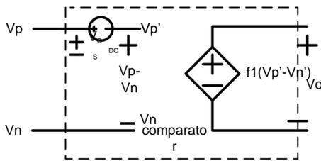
**Fig. 2.5 Model for a comparator including input-offset voltage.**
