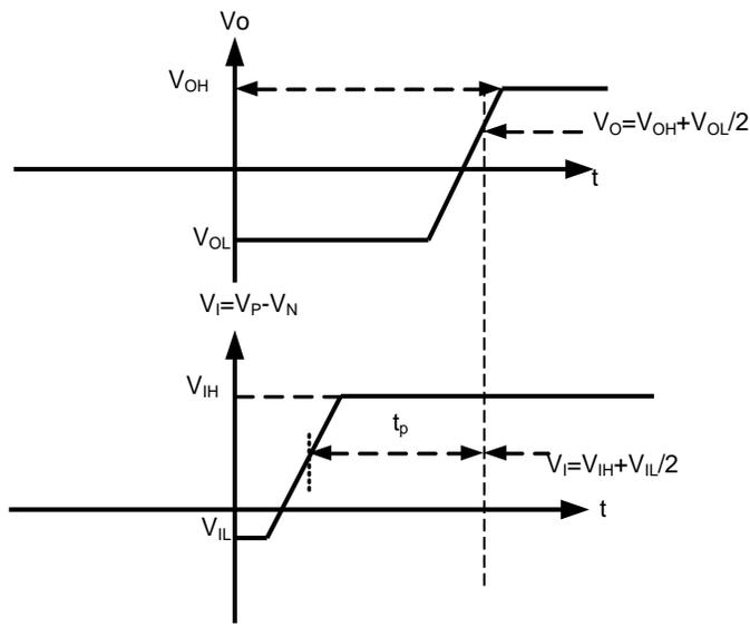
**Fig.2.7. Propagation delay time of a noninverting comparator.**
