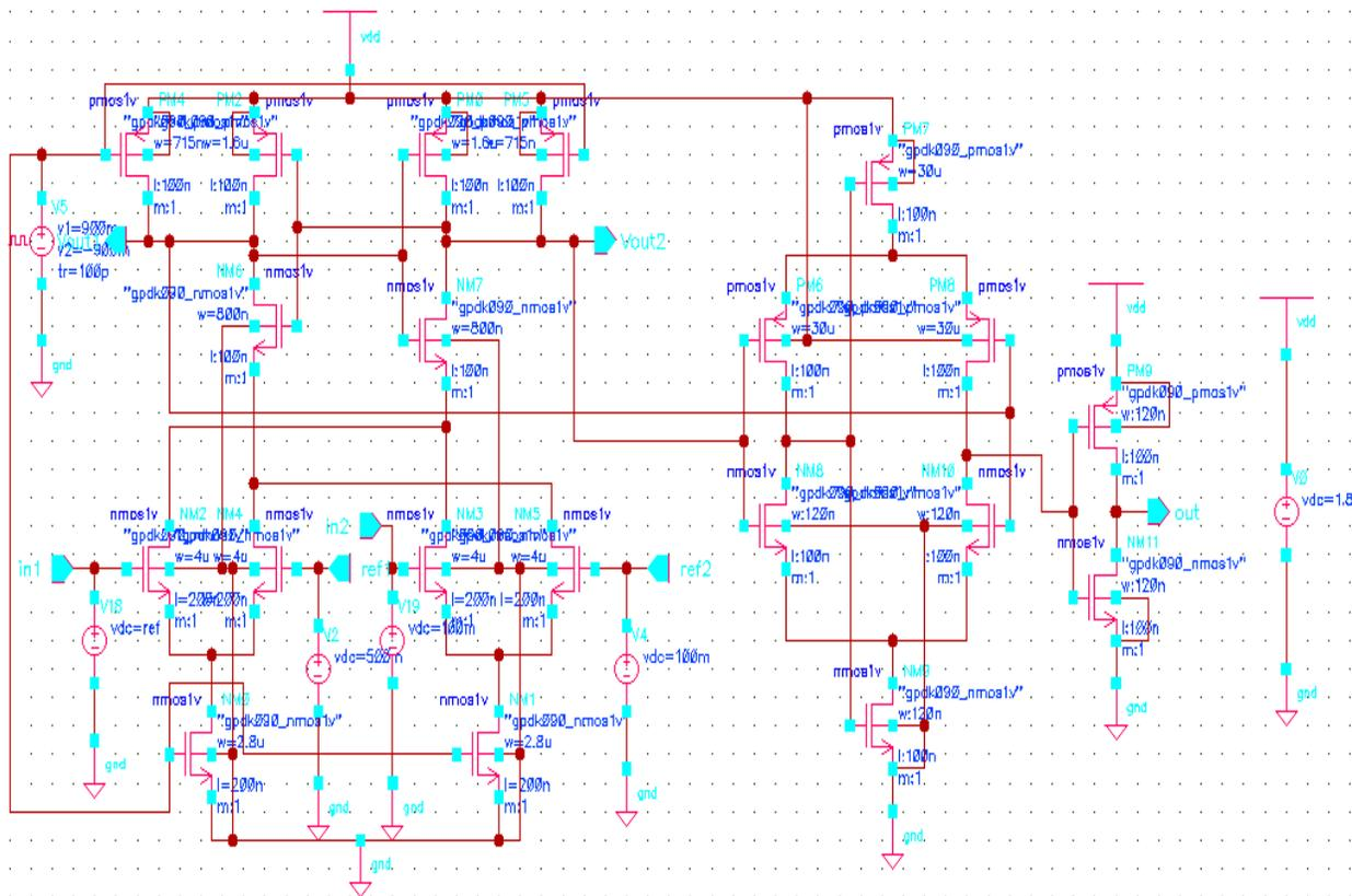
**Fig. 3.10 Differential Dynamic comparator circuit**
