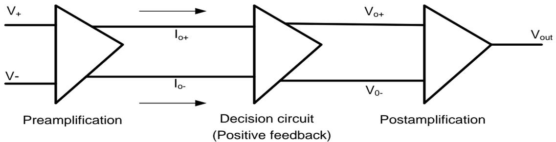
Fig. 2.8 Block diagram of Comparator
