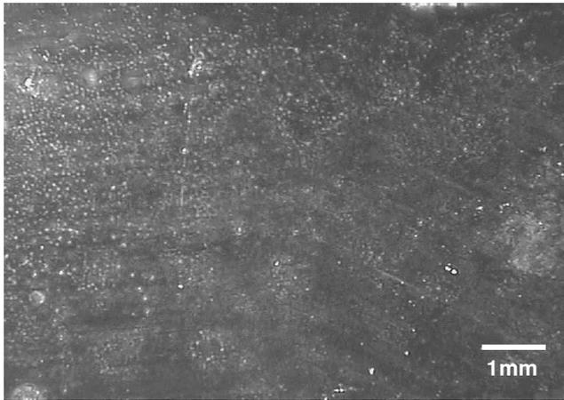
**Fig. 1** Typical surface morphology of the HPDL-fired enamel glaze on the mild steel (2 kW/cm<sup>2</sup> power density, 480 mm/min traverse speed)
