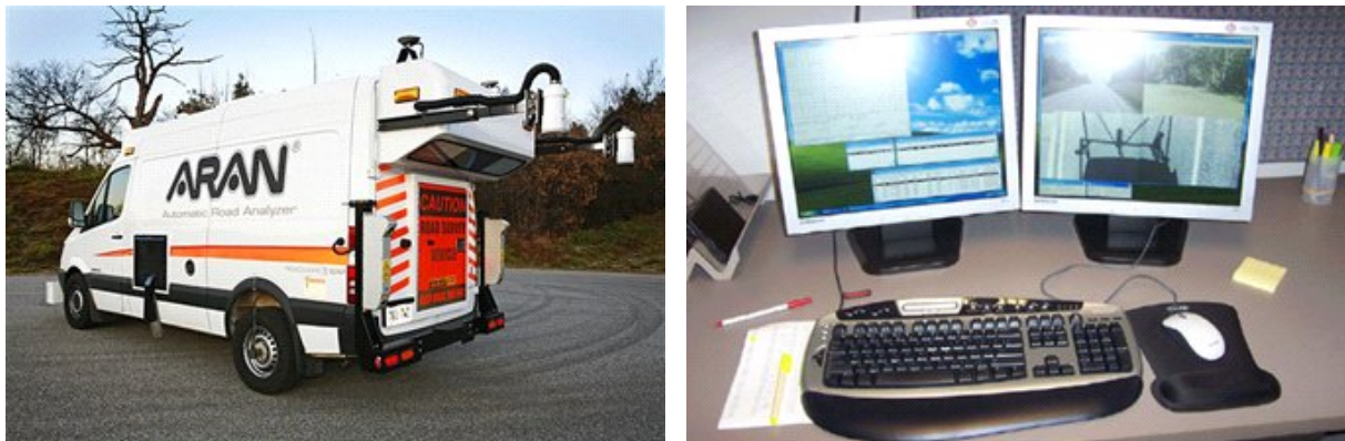
Fig. 1: Pavement inspection vehicle ARAN (Fugro Roadware 2010) and manual assessment workstation (MnDOT 2009).
