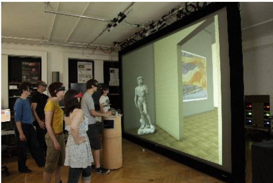
Fig. 1: The six-user display. Each user is tracked and perceives a separate stereoscopic image.
