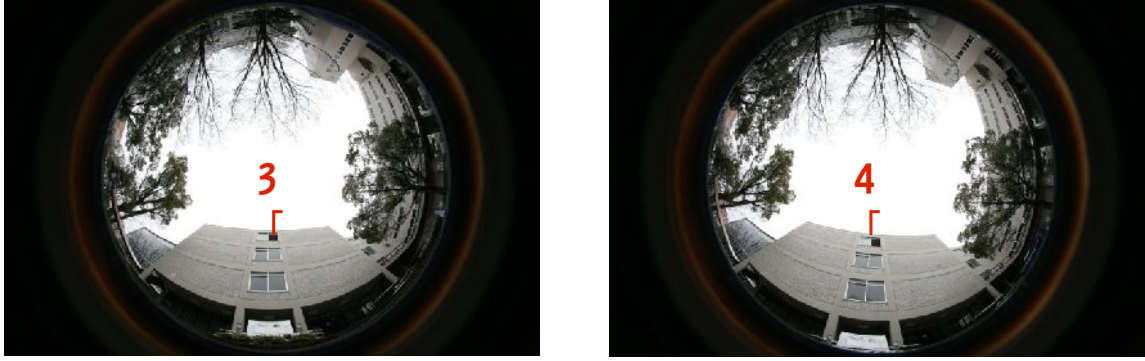
Fig. 12: Captured iamge pair #2: The camera heights are 0.53m (left) and 1.29 m (right). The red points, #3 and #4 are the corresponding points to be targeted.
