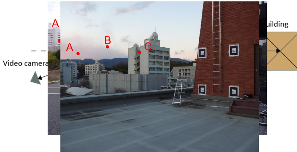
Fig. 3 (b): The building of which distance to the set of the markers ( k ) is 123m and its measuring points.
