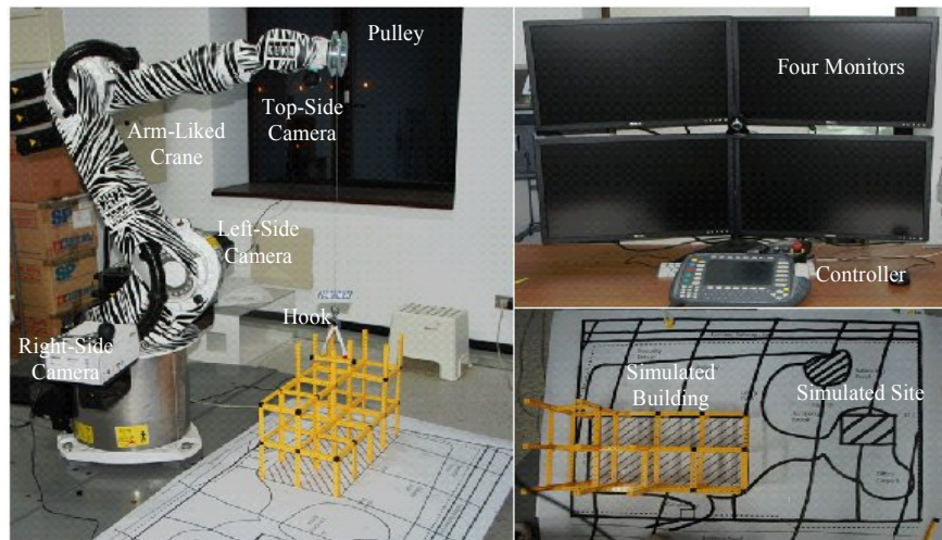
Fig. 6: Tele-operated crane prototype: (a) an overview, (b) remote cabin, and (c) simulated steel structures.
