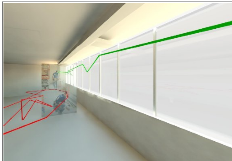
Fig. 9: Augmenting the BIM model with picture of workers and the traces of their movement
