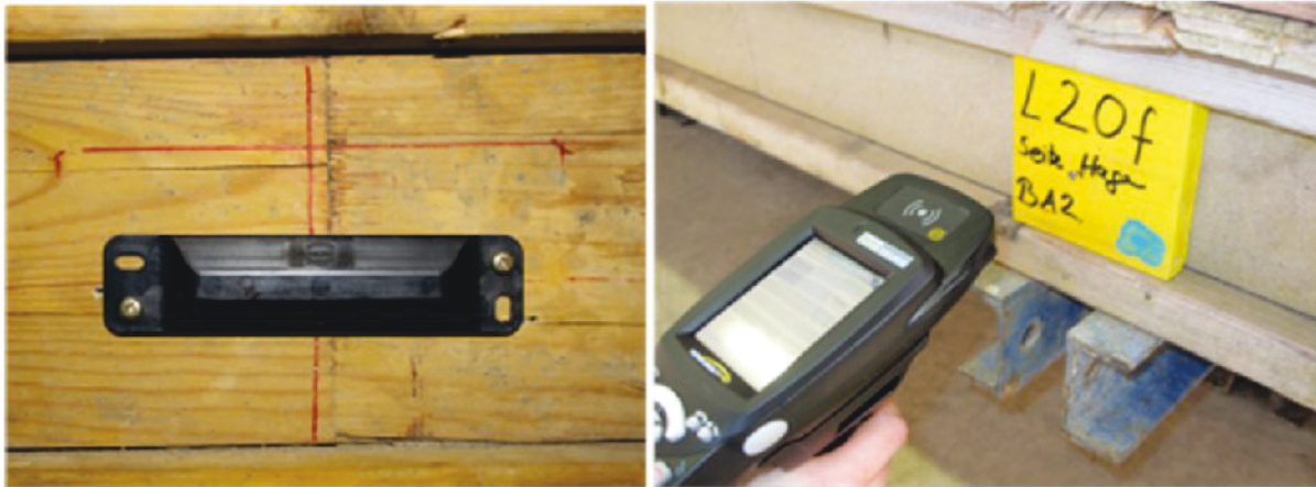
Fig. 6: Labeled modular shuttering systems (hard tag on the left, Smart Label on the right)
