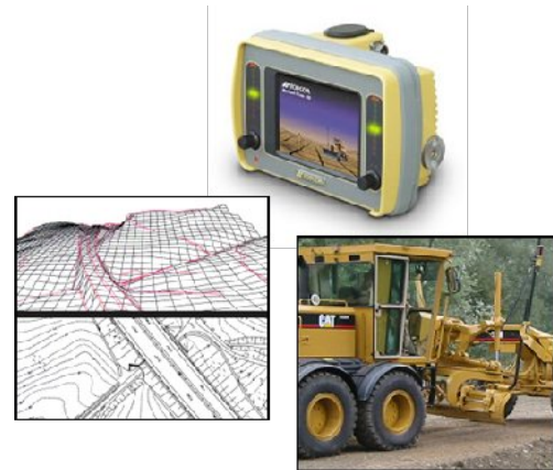
Fig.9: Control and reporting of “As Build” data by on side GPS / WLAN technology (source: TOPCON, RIB AG)
