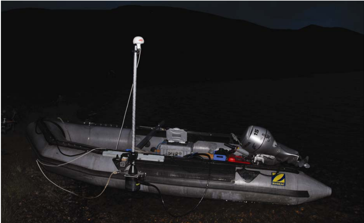
Figure 4: A hydroacoustic system assembled and installed on a small survey vessel in preparation for a night-time survey of a lake. The system's grey surface unit can be seen in the middle of the vessel, with an open ruggedised laptop on top of it and a blue 12 volt battery to its stern. The system's transducer hangs over the vessel's port side at the lower end of a pole topped by a GPS unit and which is lowered prior to survey in order to place the transducer's face approximately 0.5 m below the water level.
