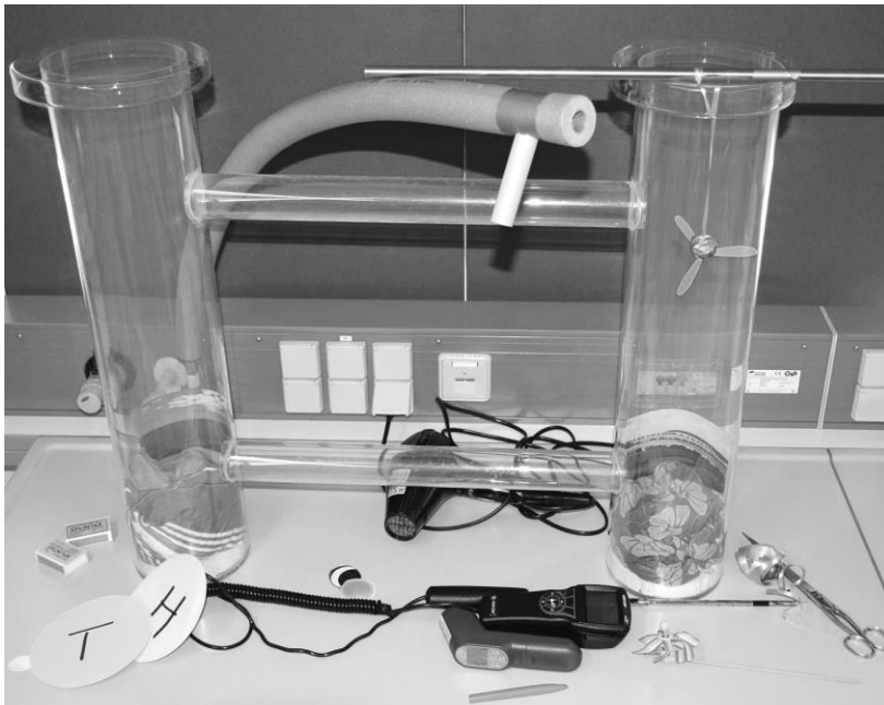
Figure 4. Airstream model, enabling thermally, dynamically or orographically induced airstreams to drive propeller (own photograph).
