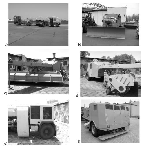
Photo 7. Cleaning set: a) a cleaner with a tractor unit with no snowplough attached,b) a cleaner with a tractor unit with a snowplough attached, c) a brush, a front view,d) a brush, a side view, e) a blower, f) a magnetic plate
