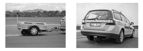
Photo 8. Examples of devices for the measurement of the friction coefficient: a) towed with a vehicle, b) attached to a car Source: websites of manufacturers.
