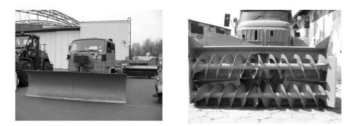
Photo 4. Airport snowploughs: a) 4-metres ordinary mouldboard snowplough, b) snow cutter Source: the author's own collection.
