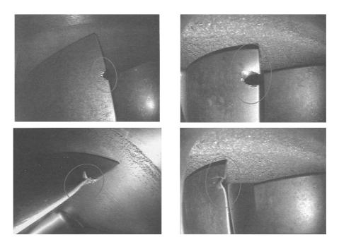
Photo 1. Damage to the blades of a MIG-29 compressor after sucking contamination Source:  $48^{th}$  Conference of the Safety of the Polish Air Force Flights, Deblin 2005.
