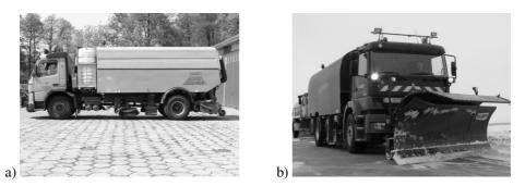
Photo 6. a) airport vacuum cleaning machine, a side view, b) airport vacuum cleaning machine with a snowplough attached Source: a - the author's own collection, b - 31<sup>th</sup> Air Base.
