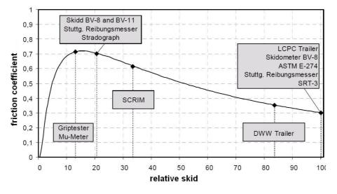
Fig. 2. Diversification of the methods of measuring the friction coefficient with exemplary measurements<sup>18</sup> Source: http://www.gddkia.gov.pl
