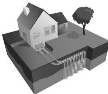
Figure 3 – The outer loop heat pump vertical type
