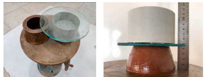
Fig. 10. Representative images showing details of the buildability test.
