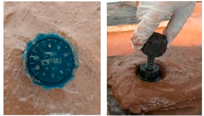
Fig. 8. Representative images showing the details of vane shear test.
