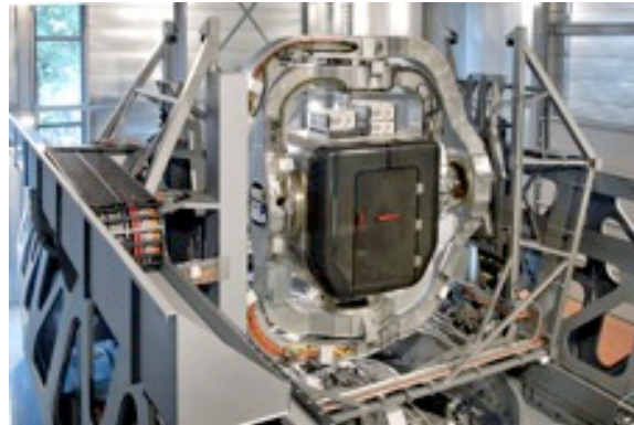
Figure 4. Six-degrees-of-freedom plus continuous-G motion system of Desdemona flight simulator. Image courtesy TNO.
