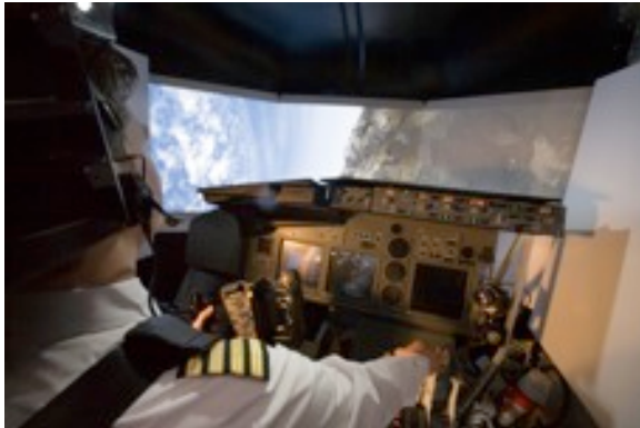
Figure 3. Transport airplane cockpit configuration of Desdemona continuous-G flight simulator. Image courtesy TNO.
