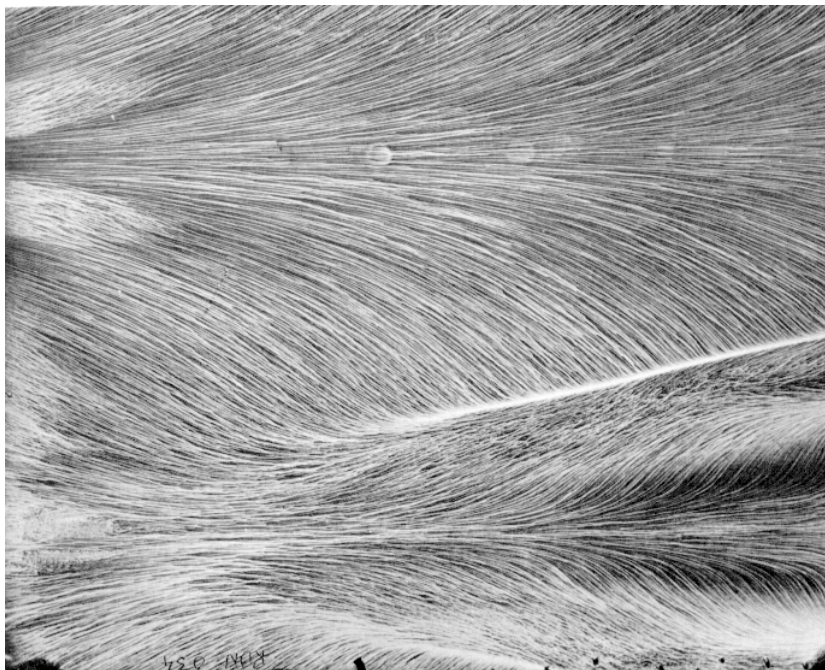
Figure 16a. Oil flow picture of the flow over a blunted cylinder under incidence.
