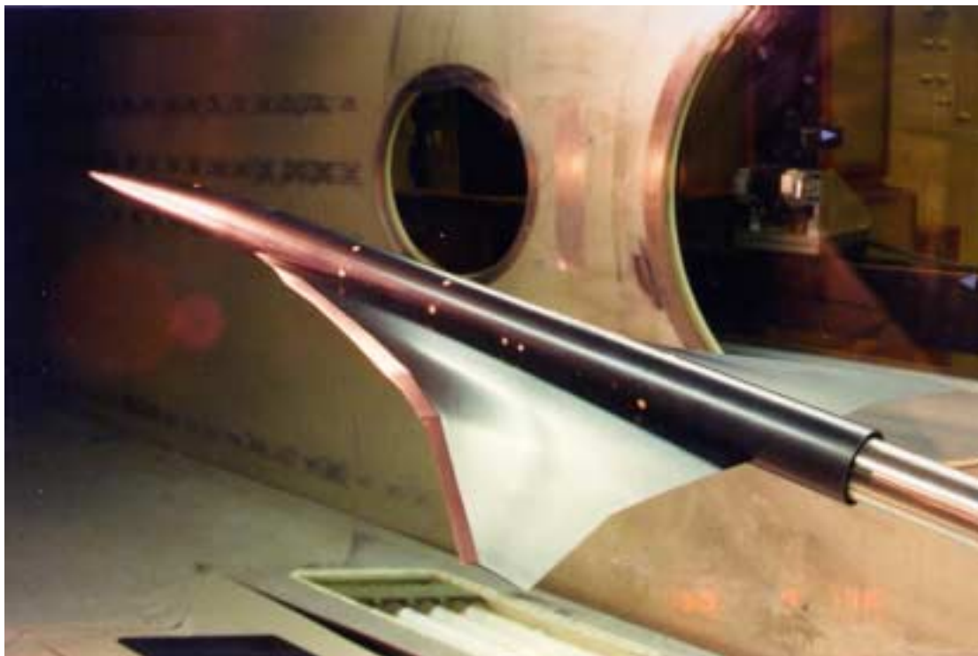
Figure 19. The EUROSTAR model with low speed wing in the test section of the DNW-HST; the deflected leading edge is clearly visible.
