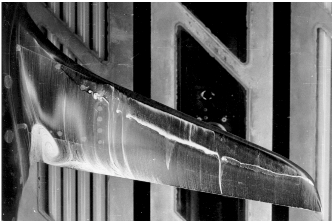
Figure 18. Oil flow pattern on the first supercritical wing designed by NLR showing a spiral type separation at the wing root (DNW-HST test results).
