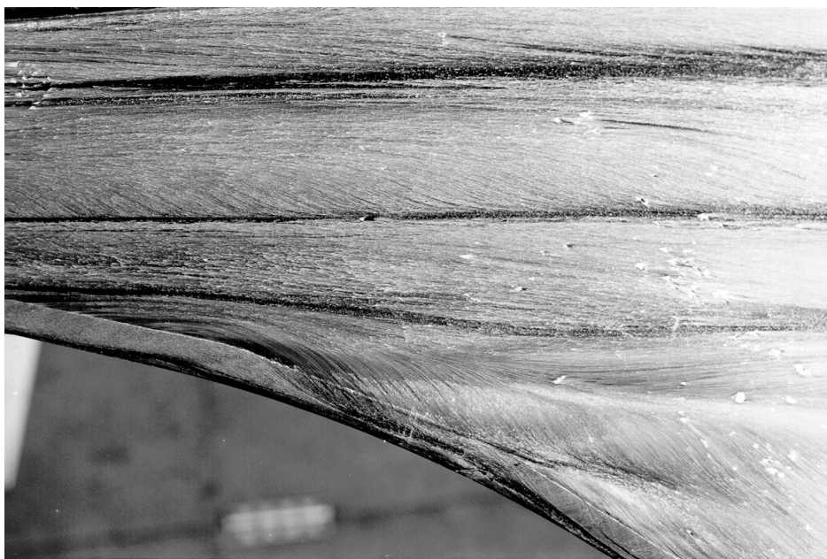
Figure 20. Oil flow pattern of the flow for the EURO SUP model close to the low speed design condition; (a) gives an overall view and (b) a close-up of the leading edge near the kink location showing a local separation; the dark lines are indicative of vortices that are embedded in the flow.
