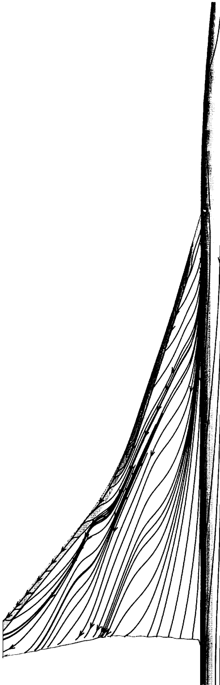
Figure 22. Surface flow as calculated with a Navier-Stokes code showing a tendency of streamwise vortices to develop in addition to the separation in the leading edge kink region (calculations made by Van Muijden of NLR as part of a GARTEUR activity).
