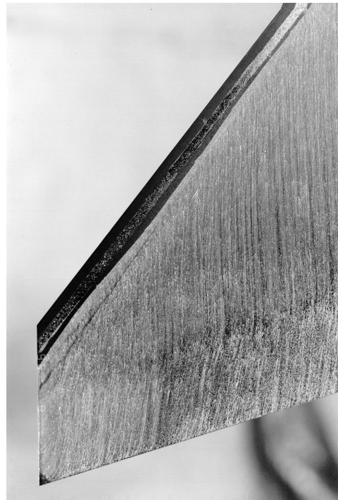
Figure 18b: Detailed view of outer wing upper side oil flow pattern at the transonic design condition
