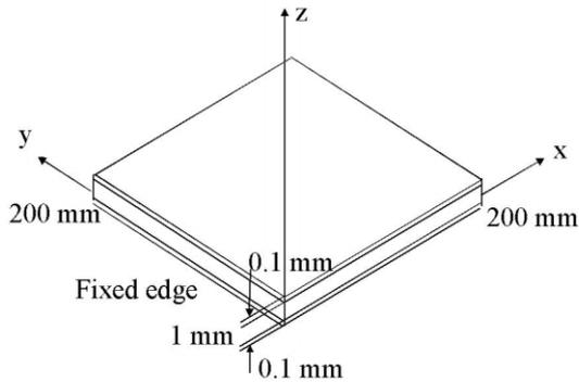
**Figure 3** A laminated composite plate with piezoelectric layers.
