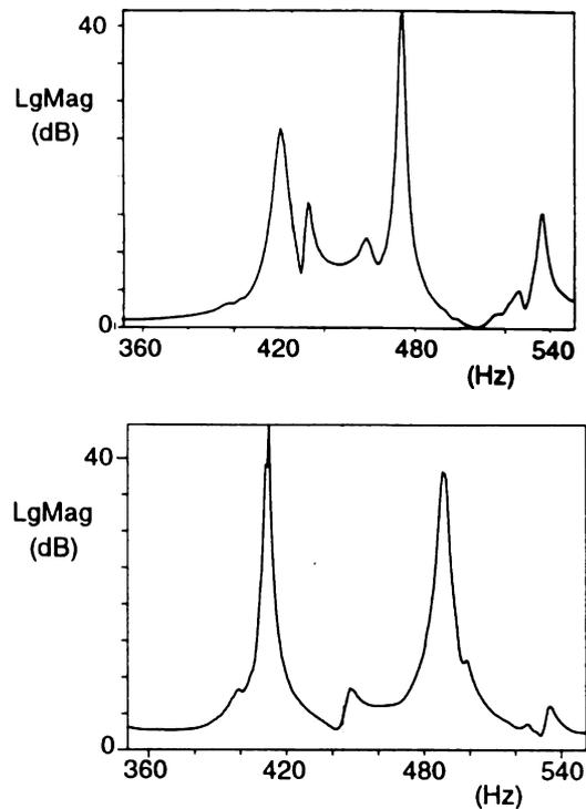
**Figure 5** FRF in a point of the plate with tuned dampers in the initial positions (upper) and the optimized positions (lower).
