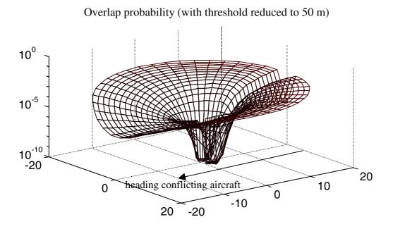
Figure 6: Overlap probability (z-axis) with threshold reduced to 50 m is represented for various path angles and times to minimum predicted separation (horizontal axis).
