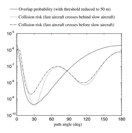
Figure 11: Difference between situations in which a faster aircraft crosses before or after a slower aicraft. Evaluated overlap probability (with threshold reduced to 50 m) and collision risk are shown.
