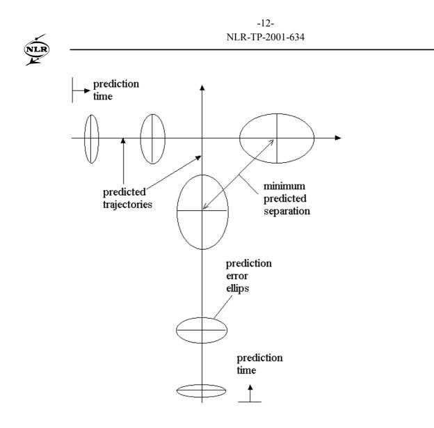
Figure 1: ATM example in the horizontal plane.
