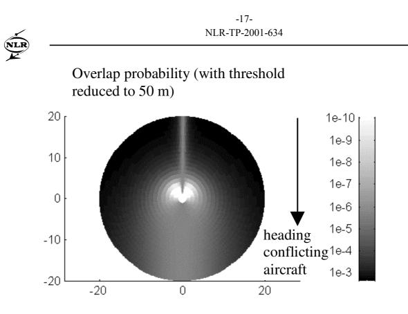
Figure 7: Overlap probability (with threshold reduced to 50 m) is represented by colours for various path angles and times to minimum predicted separation.
