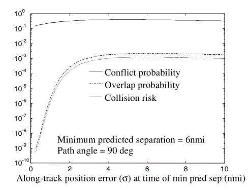
Figure 4: Conflict probability, overlap probability (with threshold reduced to 50 m) and collision risk in example 1 (log scale).
