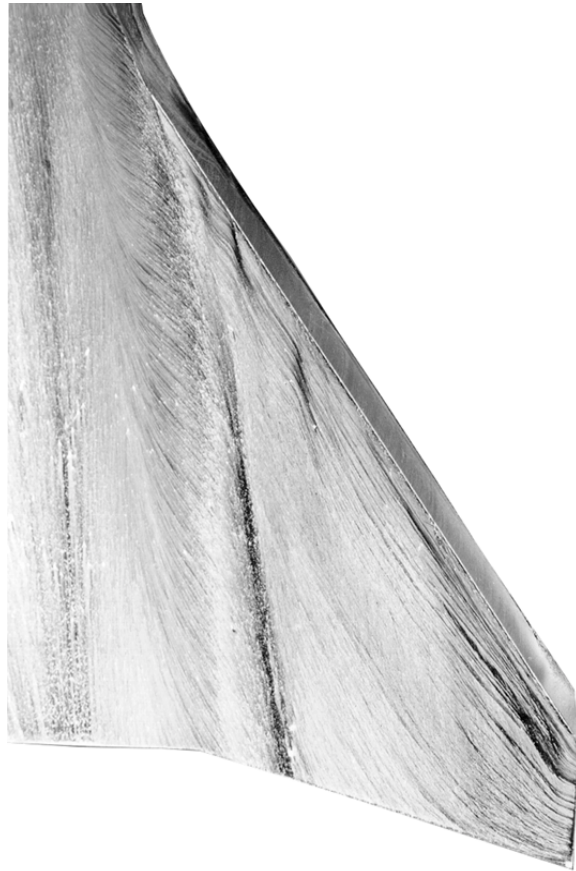
Fig 12b Outer wing oil flow visualisation at \alpha = 10 degrees
