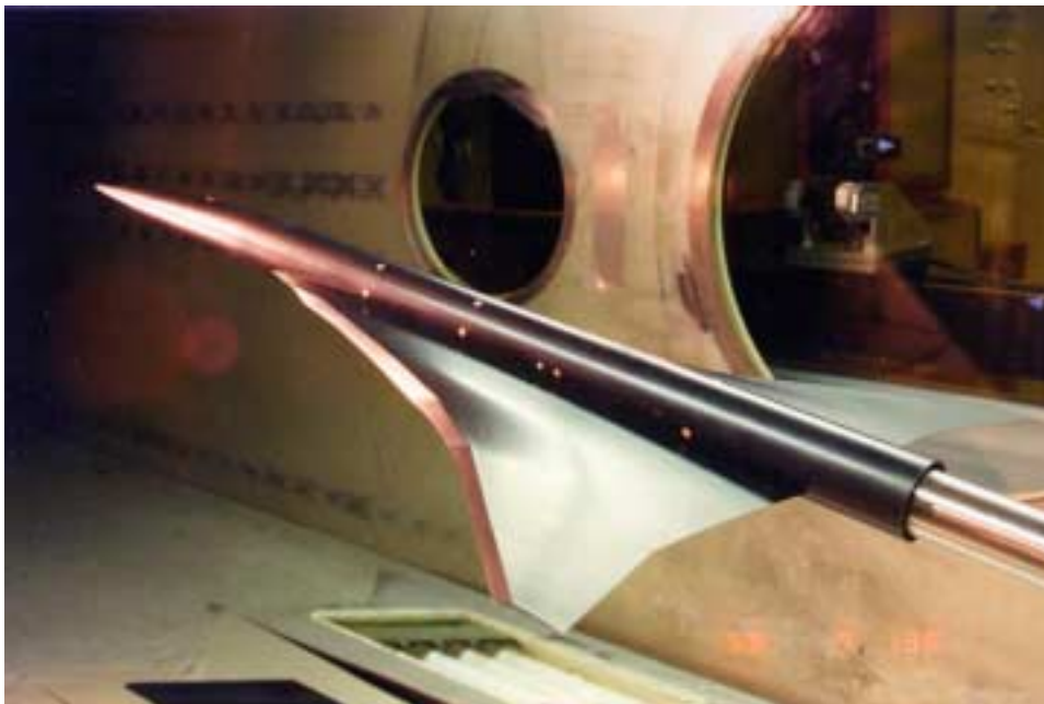
Fig 1 Wind tunnel model of low-speed configuration, showing deflected leading-edge flaps
