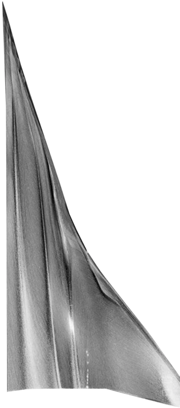
Fig 12a Oil flow visualisation at \alpha = 10.5 degrees
